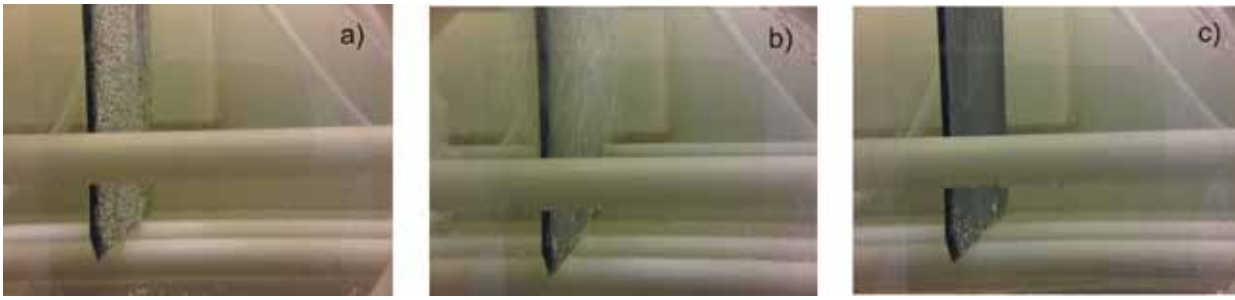
Figure 3. Texturing of a mono-Si wafer in a KOH-IPA etching solution by using a closed etching bath in which vacuum steps are applied: (a) a mono-Si wafer covered by hydrogen bubbles (vacuum off), thus slowing down the etching process on this wafer; (b) the same wafer, with hydrogen bubbles detaching from the surface when a short vacuum-process step (vacuum on) is applied; (c) a picture taken immediately after the vacuum step in (b), showing the wafer to be almost free of hydrogen bubbles (vacuum off), and therefore allowing the etching process to accelerate again. The vacuum steps are applied periodically during the etching process – by doing this, the etching time is considerably reduced.
