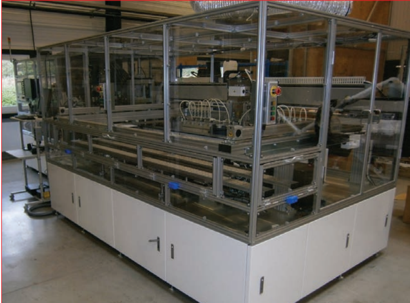
Figure 8. Automated tabber-stringer system for back-contact cells, including paste dispensing, glass fibre fabric lay-up, hot air soldering, and EL testing of the fabricated strings.
