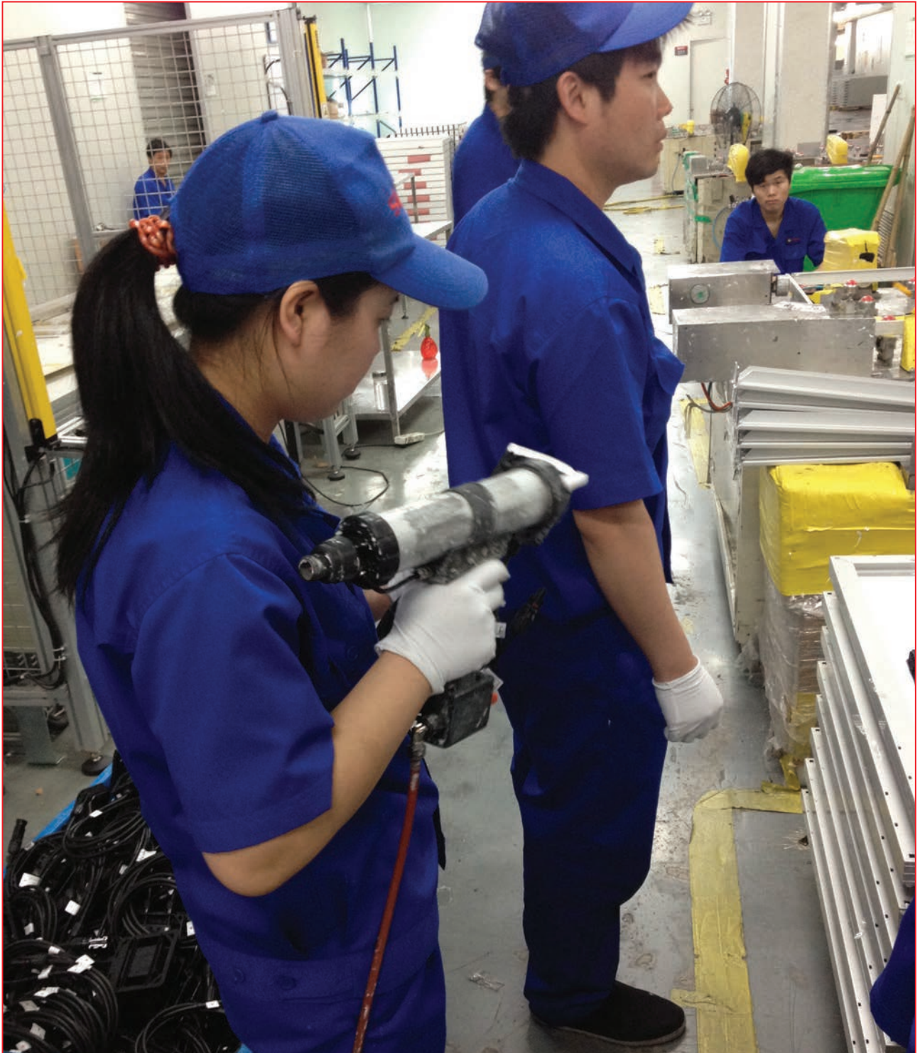
Figure 2. Incorrect handling during a junction box sealing operation.
