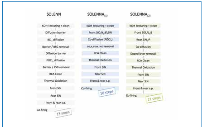
Figure 3. The n-PERT process flow simplifications: gaseous diffusion route (SOLENN), co-diffusion \text{SiO}_x\text{N}_y\text{:B}/\text{POCl}_3 route (SOLENNA (1) ) and full dielectric co-diffusion route (SOLENNA (2) ).
