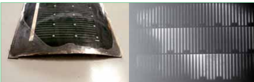
Figure 5. Effects of moisture ingress due to adhesion loss: delamination (left), and degradation as indicated by an electroluminescence image of a mini-module (right).
