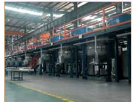
Figure 2. Jinggong assembly line for the JLL500N Si ingot furnace.
