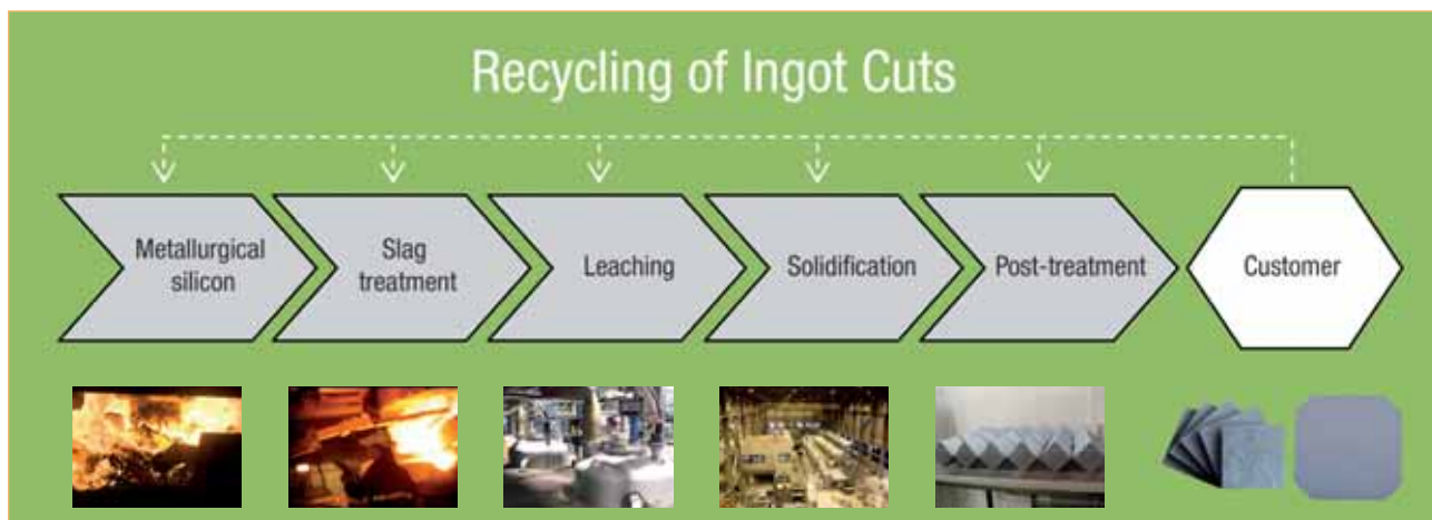
Figure 1. The five steps in the metallurgical route industrialized by Elkem: reduction furnace, slag treatment, leaching, one-directional solidification and post-treatment. The robustness and flexibility of the process in terms of handling recycled ingot cuts is highlighted.
