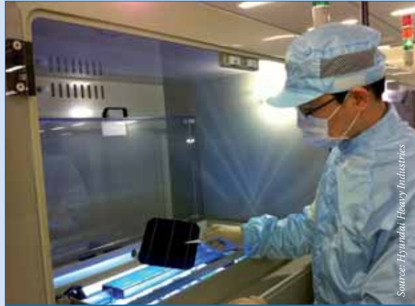
HHI researchers have been working on improving the LDSE technology with the addition of copper contacts on the front of the cell.
