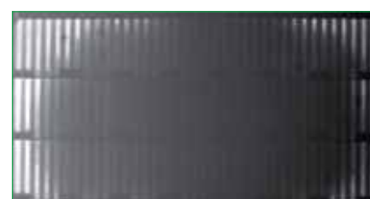
Figure 9. Electroluminescence image of a mini-module showing degradation caused by moisture ingress through the front barrier film.
