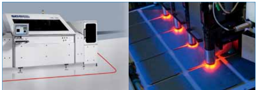
Figure 2. Inkjet system (left) including loading/unloading section. Alignment system (right) recognizes wafer position for accurate placement of the printed mask.
