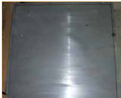
Figure 1. Cross section of Jinggong's mono-like crystalline ingot (height 100mm).
