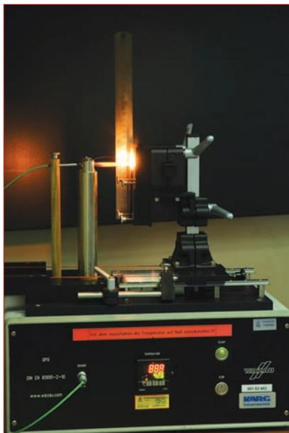
Figure 2. Glow-wire test: test for resistance to ignition.
