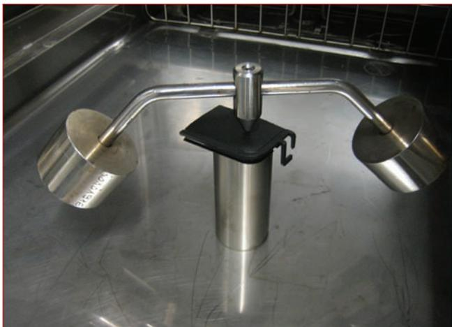
Figure 1. Ball pressure test: material test for resistance to heat.
