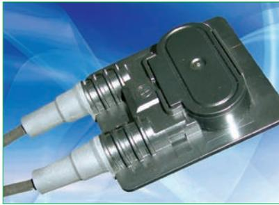
**Yamaichi Electronics' thin-film junction box uses kink protection with Hermetic Sealed technology**
