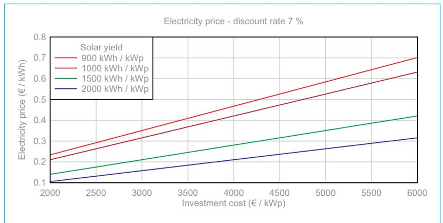
Figure 6. Electricity price for 7% discount rate and 20-year system lifetime for different yield rates.
