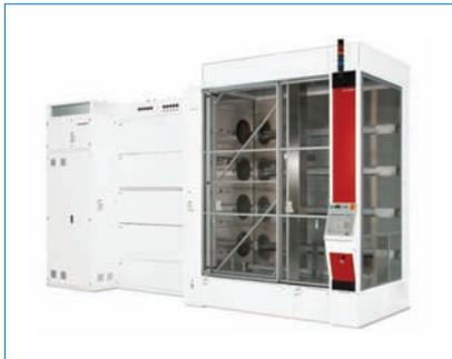
centrotherm's batch-type system for nitride deposition in c-Si solar cell processing.
