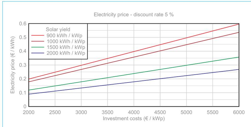
Figure 4. Electricity price for 5% discount rate and 20-year system lifetime for different yield rates.
