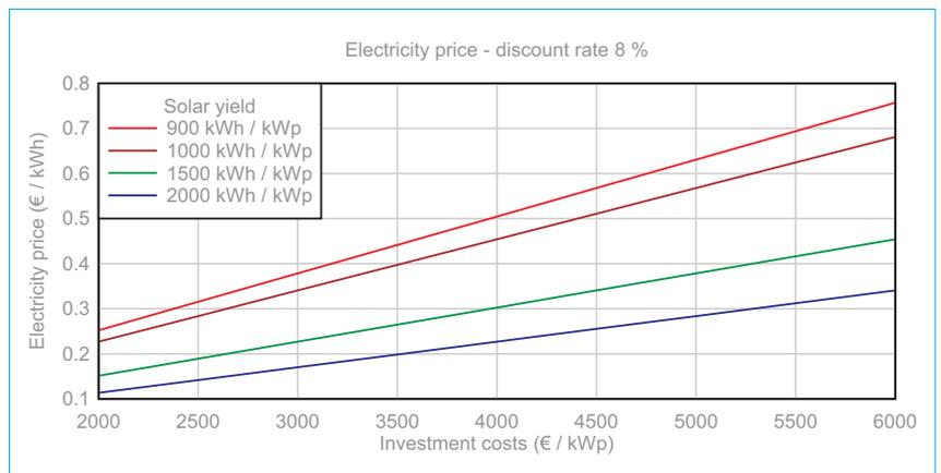
Figure 7. Electricity price for 8% discount rate and 20-year system lifetime for different yield rates.
