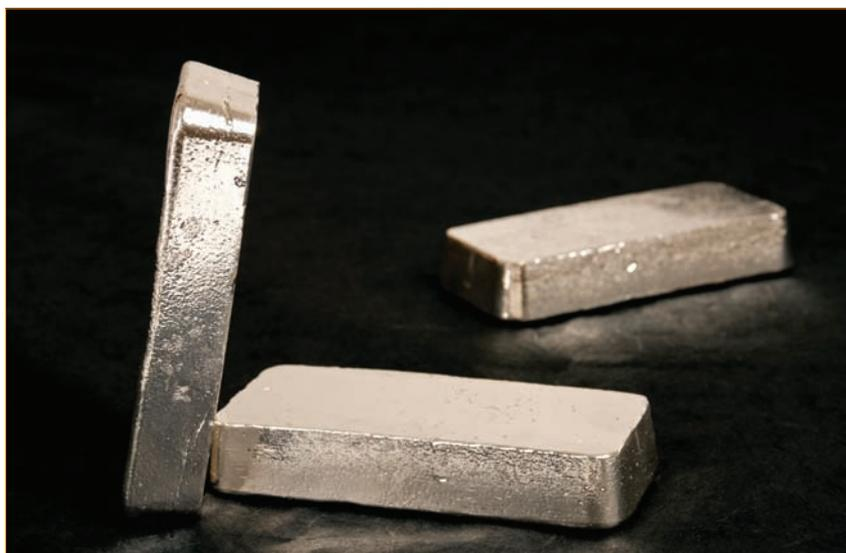
**Figure 2. Silver's unique properties as a highly conductive metal that forms stable connections to crystalline silicon means it is very hard to replace with another single material.**
