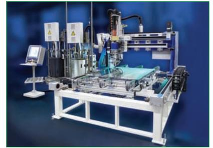
**Bystronic's photovoltaic-TPA system offers continuous encapsulation and sealing of thin-film modules**
