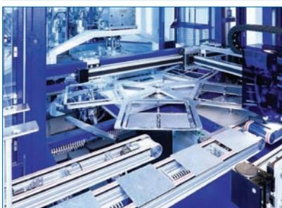
**ICP-PECVD tool from Singulus enables development of passivation layers for new cell concepts**
