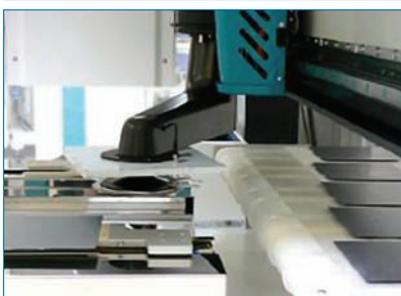
**SpeedPicker 1.1 from Manz offers throughput rate of 5,000 wafers per hour using carbon arms**
