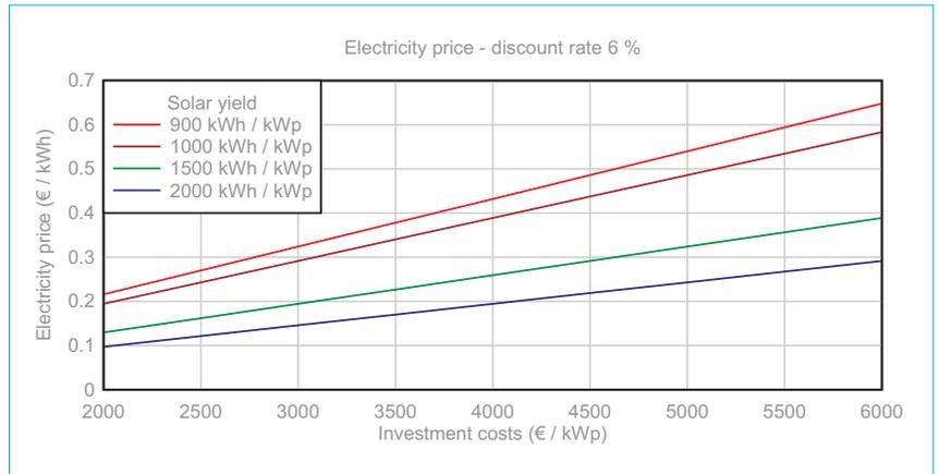
Figure 5. Electricity price for 6% discount rate and 20-year system lifetime for different yield rates.
