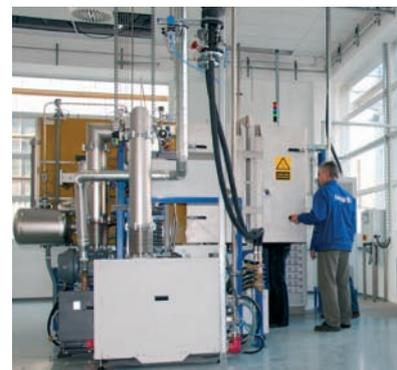
PE-CVD reactor for thin layers.
