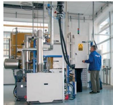
PE-CVD reactor for thin layers.
