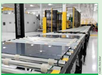
First Solar is introducing new production lines to manufacture its 400W large-area 'Series 6' modules.
