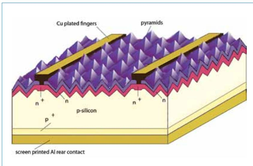
Figure 1. Standard single-sided LDSE solar cell, showing laser-doped selective emitter front surface with plated metallization and screen-printed rear Al BSE.
