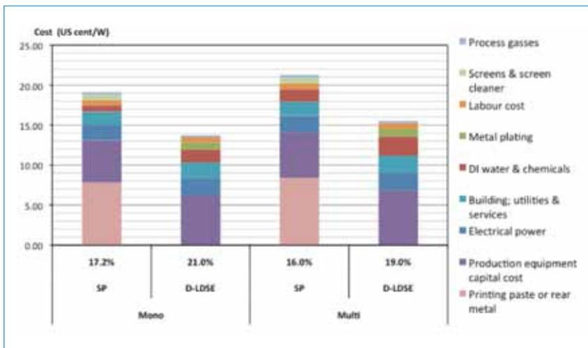
Figure 7. Cell conversion cost of ownership for D-LDSE solar cells compared to that of standard screen print solar cells. Significant savings are realised due to much higher efficiencies and elimination of screen print processes and metal pastes.
