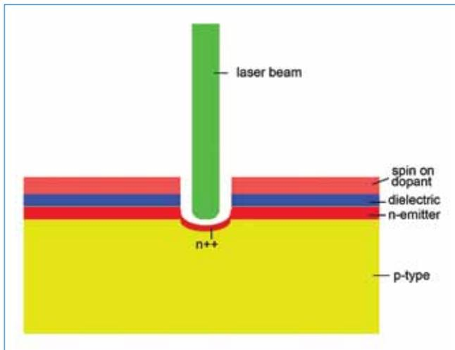
Figure 2. The laser doping process. The dielectric layer is removed while a dopant source is incorporated into the molten silicon, forming a selective emitter and plating mask in one step.
