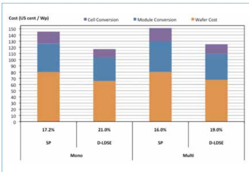
Figure 8. Overall cost of ownership for LDSE solar cells compared to that of standard screen print solar cells, showing very significant savings in wafer and module conversion costs.
