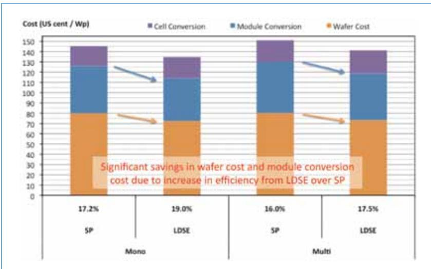
Figure 4. Overall cost of ownership for LDSE solar cells compared to that of standard screen print solar cells. Savings in wafer cost and module conversion due to higher power density are realised.
