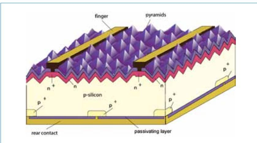
Figure 5. Double-sided LDSE solar cell, showing laser-doped selective emitter front surface and passivated, locally diffused rear surface with point contacts.
