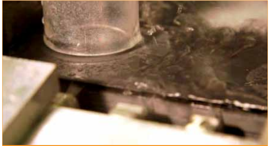
Figure 6. Compressed air is used to clear the signal path of the distance sensors.
