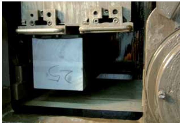
Figure 2. Wafers in a wire saw (left). After sawing, the wafers are clustered into packages (right).
