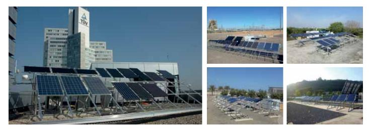
Figure 1. The test sites operated by TÜV Rheinland for PV module characterisation and energy yield measurements (clockwise from left): Cologne (Germany, moderate climate), Tempe (Arizona, dry continental climate), Chennai (India, tropic climate), Thuwal (Saudi Arabia, dry desert climate with sand deposition) and Ancona (Italy, Mediterranean climate).
