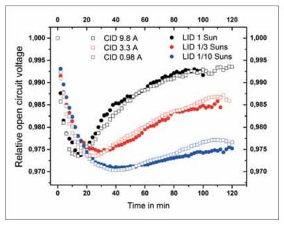
Figure 5. Comparison of LID and CID for different intensities at 140°C on borondoped Cz silicon solar cells showing B-O LID [16] treatments can also be carried out, such as illuminated annealing or a second firing step. However, these approaches are lavish and have several disadvantages i.e. no complete avoidance or avoidance to an unknown extent and negative influences on the solar cell efficiency and other parameters.
