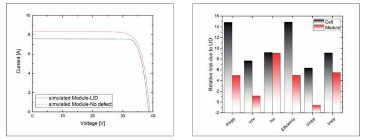
Figure 3. Electric simulations of module parameter losses when 12 cells in a 60-cell standard module show significant LID. Left: IV-curves of a module before and after LID. Right: Relative changes in electrical characteristics of cell and module after light induced degradation
