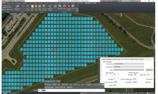
PVCAD combines the main attributes of AutoCAD design software with solar modelling capabilities
