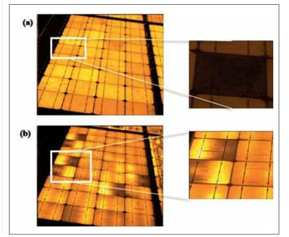
son between (a) DPL image (contrast adjusted) and (b) DEL image captured for a PV module on-site in a 10-year old PV system in Singapore
