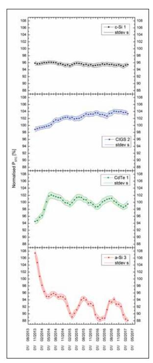
Figure 4. Monthly averages of STC-corrected nominal power for four PV module types, normalised to stated nominal power, for the Ancona test site in Italy (uncertainty:  $\pm 2.5\%$ )
