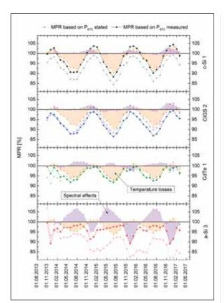
Figure 5. Monthly module performance ratio based on stated  $P_{\text{STC}}$  for four PV module types, compared with the MPR based on monthly measured  $P_{\text{STC}}$  for the Ancona test site in Italy. A deviation from 100% means yield losses or gains; the temperature (orange) and spectral effect (purple) contributions are indicated
