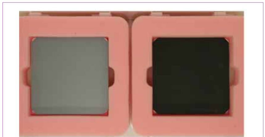
Figure 2. Pyramidal texture etch (left) and the same type of wafer with a black silicon etch (right).
