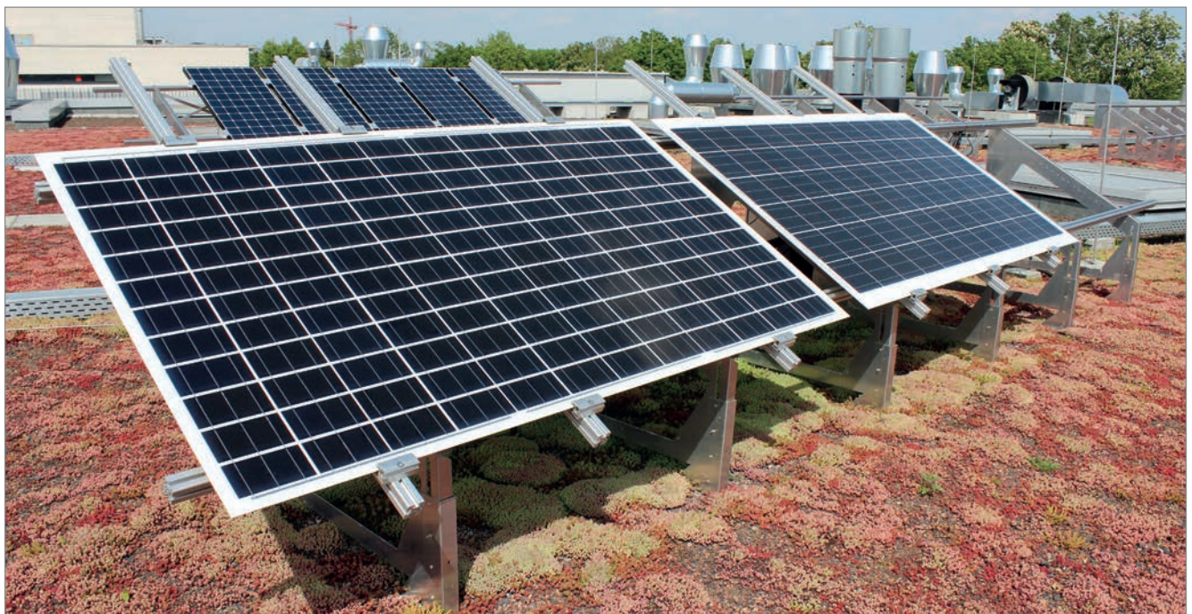
Figure 9. A half-cell module (left) and a full-cell module (right), installed at Fraunhofer CSP's ‘Outdoor PV Lab Halle’ outdoor setup.
