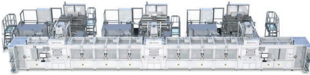
Figure 5. Meyer Burger's HELiA PECVD tool, which uses reactors based on the 'plasma box' concept. This guarantees perfect layer homogeneity, reducing contamination, and facilitates reactor cleaning [35]. Wafer carriers see only one deposition chamber, ensuring that no contamination is introduced by the carriers. (SP = screen printed.)
