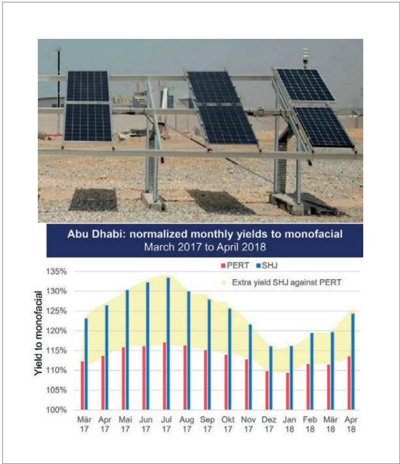
Figure 7. Field data collected from PERT bifacial modules and SHJ SWCT bifacial modules.
