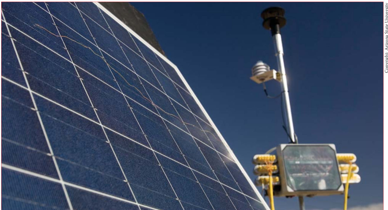
Figure 1. The ANSI/UL 1703 Temperature test is performed in ASU-PTL's test field.
