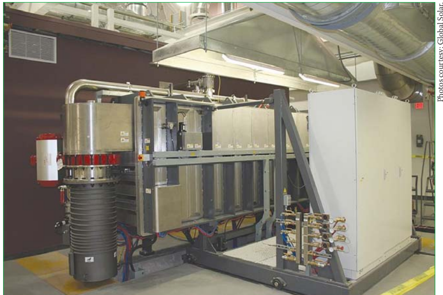
Figure 2. Global's CIGS tools use a multisource coevaporation process.
