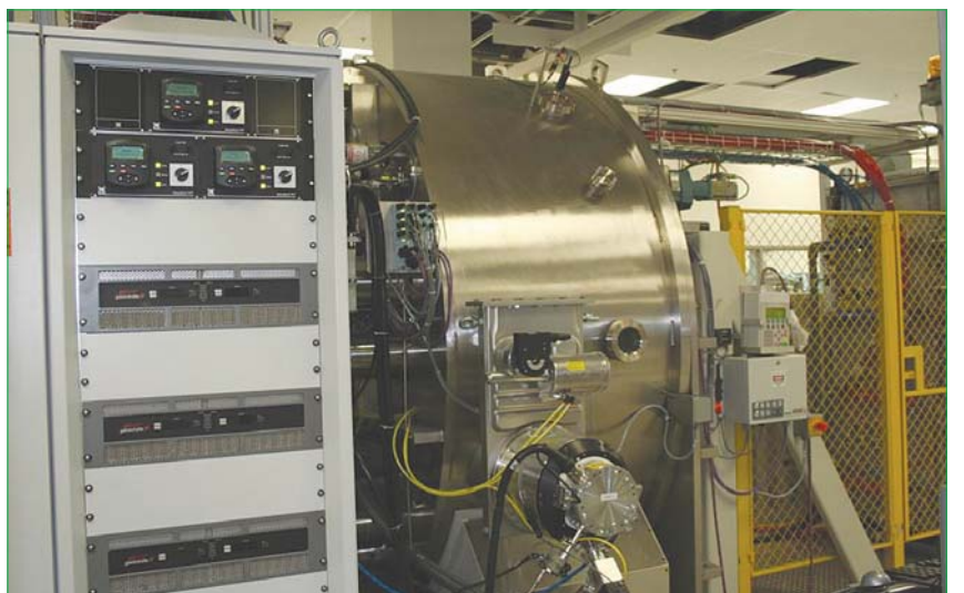
Figure 3. Large chambered systems sputter the TCO films.
