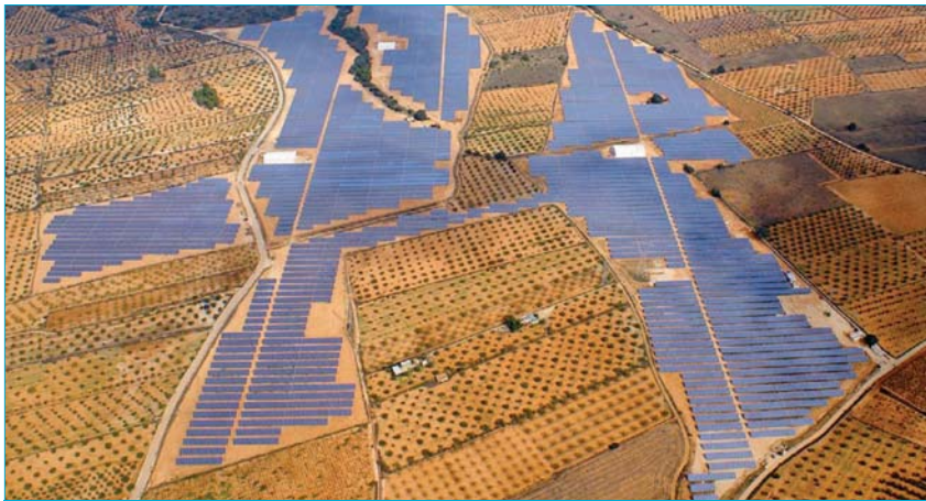
Figure 2. The Solar Park in Beneixama, Spain. In an area of 500,000m 2 , 30 million kilowatt hours of clean energy are produced annually.
