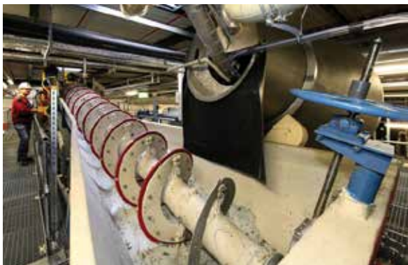
Figure 5. First Solar's first-generation recycling technology based on the mining industry's batch process
