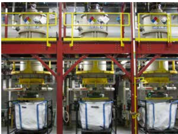
Figure 6. First Solar's second-generation recycling technology based on the chemical industry's batch process
