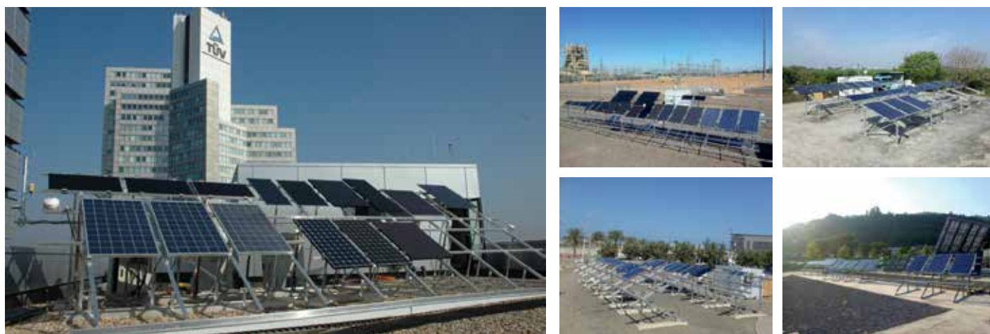
Figure 1. The test sites operated by TÜV Rheinland for PV module characterisation and energy yield measurements (clockwise from left): Cologne (Germany, moderate climate), Tempe (Arizona, dry continental climate), Chennai (India, tropic climate), Thuwal (Saudi Arabia, dry desert climate with sand deposition) and Ancona (Italy, Mediterranean climate).
