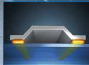
Bonding of back rails
