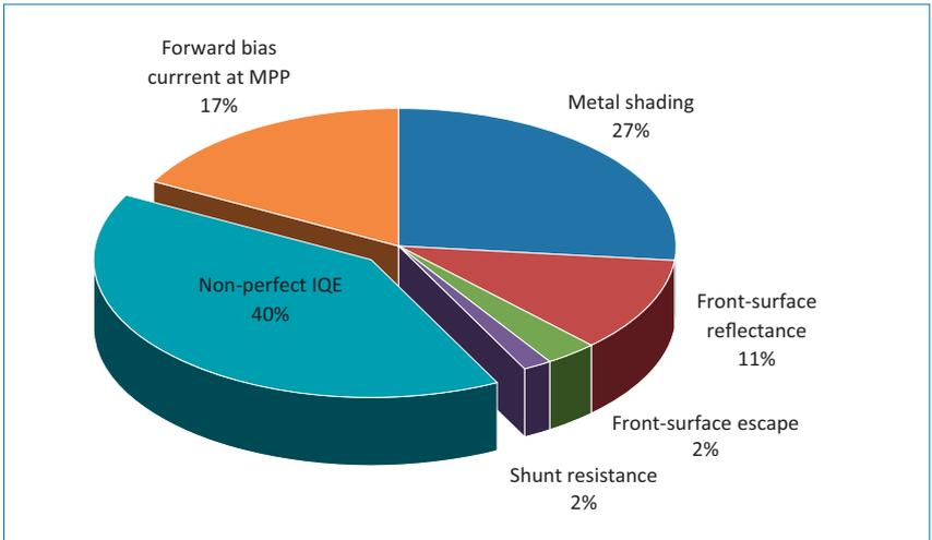
Figure 4. Pie chart of the relative current losses at the maximum power point for a standard industrial p-type Al-BSF solar cell. The total current losses amounted to  $12.7\text{mA}/\text{cm}^2$  in this specific case.
