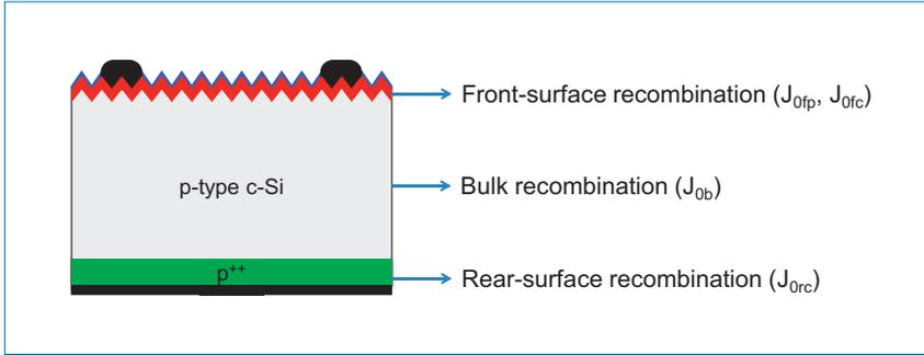
Figure 6. Sketch of a standard industrial Al-BSF solar cell, indicating the different solar cell regions which contribute to recombination losses.
