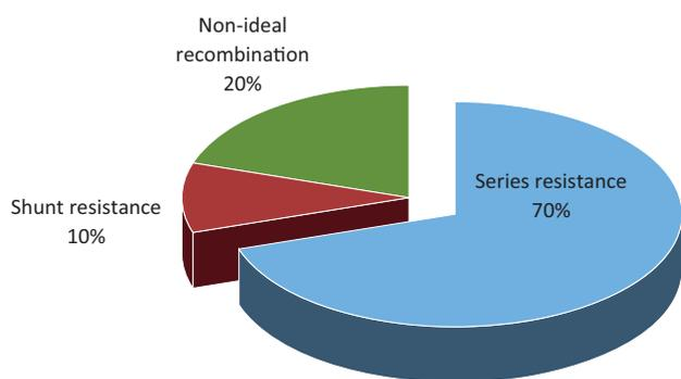
Figure 11. *FF* loss analysis of a standard industrial p-type Al-BSF solar cell.
