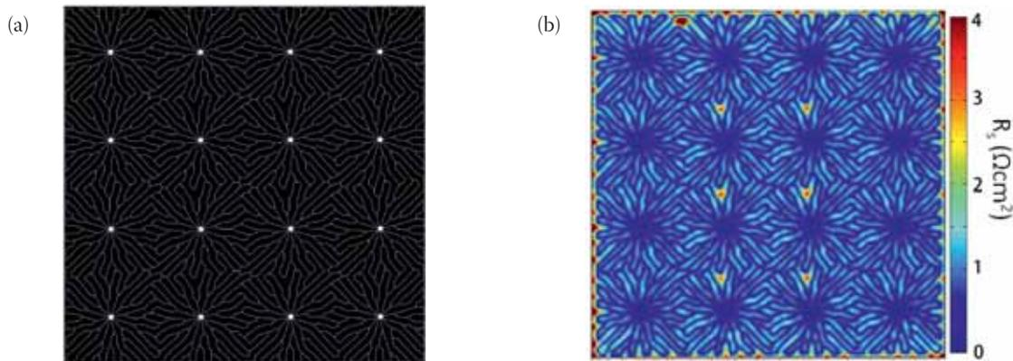
Figure 9. (a) Image of the front-side metal grid of a metal-wrap-through solar cell. (b) Corresponding local distribution of the series resistance of the solar cell under maximum power conditions, after being processed by the GRIDDLER software [10].
