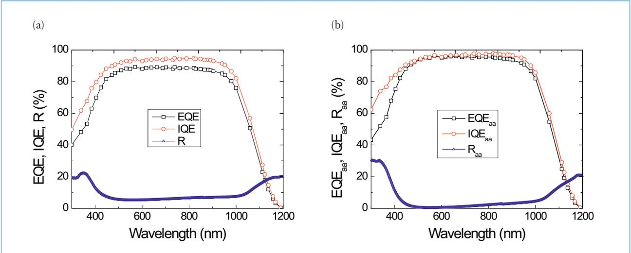
Figure 2. External and internal quantum efficiency and reflectance measurements of a standard industrial p-type Al-BSF silicon wafer solar cell: (a) full-area, and (b) active-area corrected.
