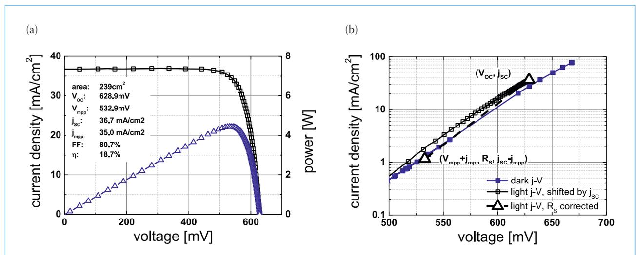
Figure 1. Current–voltage curve of a standard industrial p-type Al-BSF silicon wafer solar cell: (a) subjected to a one-sun illumination; (b) measurements taken in the dark.
