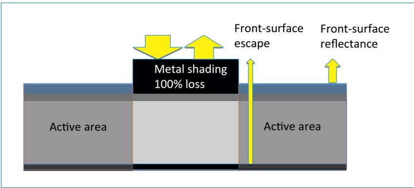
Figure 3. Schematic illustration of optical losses at the front of a silicon wafer solar cell.
