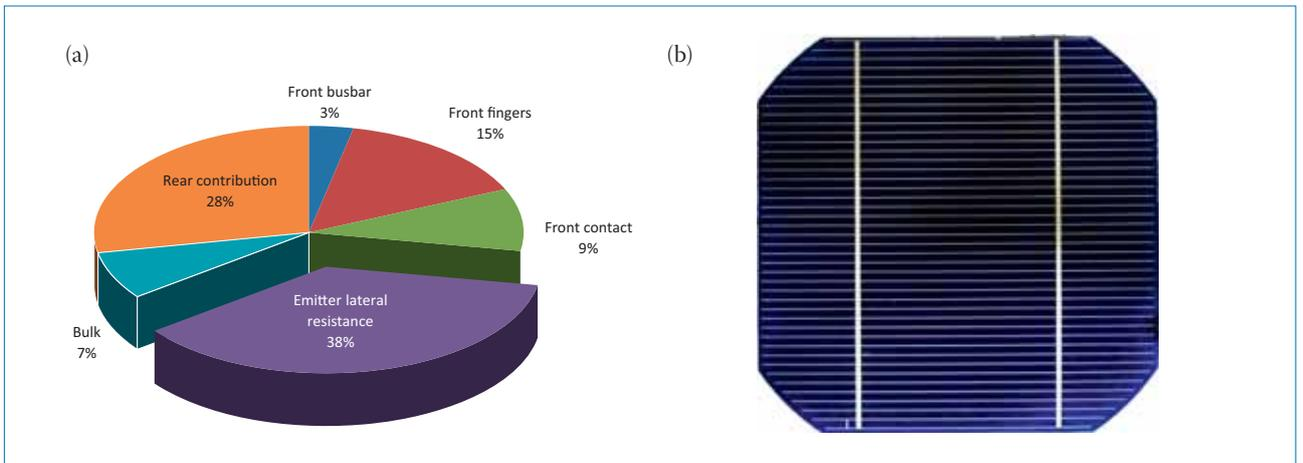
Figure 8. (a) Breakdown of measured series resistance of a standard industrial p-type Al-BSF solar cell processed at SERIS; (b) the simple H-patterned metal grid used. The total series resistance due to the front grid and the bulk were calculated to be  $0.44\Omega\text{cm}^2$ , and the remainder of the series resistance ( $0.16\Omega\text{cm}^2$  out of the total of  $0.61\Omega\text{cm}^2$ ) was attributed to the rear contact.
