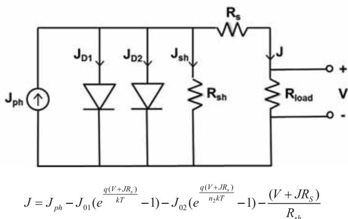
Figure 10. Two-diode model of a solar cell, and the corresponding mathematical description of the *J-V* characteristics of the cell.
