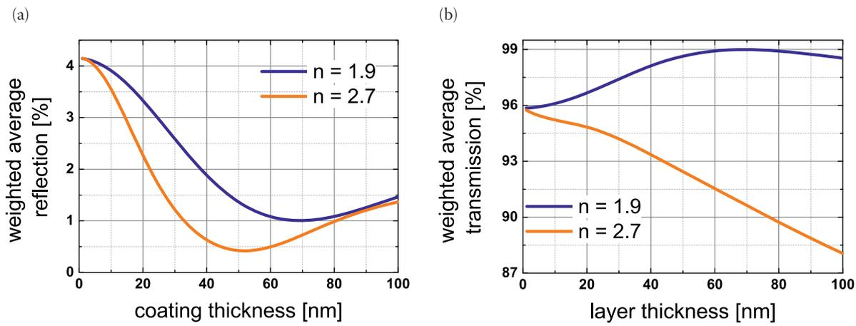
Figure 5. Investigation of two different coating materials with refractive indices  $n = 1.9$  and  $n = 2.7$  for a silicon solar cell with pyramidal texture and encapsulated with a material with refractive index  $n = 1.5$ : (a) calculated WAR, and (b) calculated WAT.
