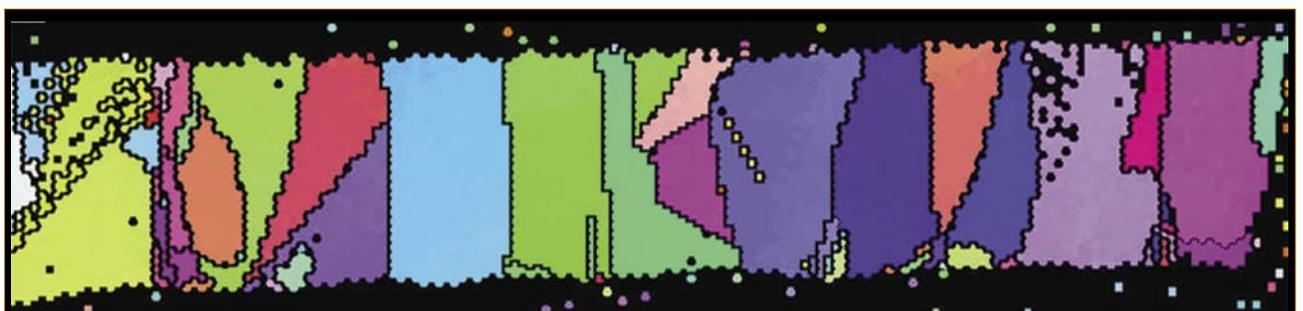
Figure 8. Cross-sectional map of crystalline orientations (black: blank). CDS Si wafers had a quite small grain size, but contained columnar grain structures and good grain boundaries, elements that are suitable for solar cells.
