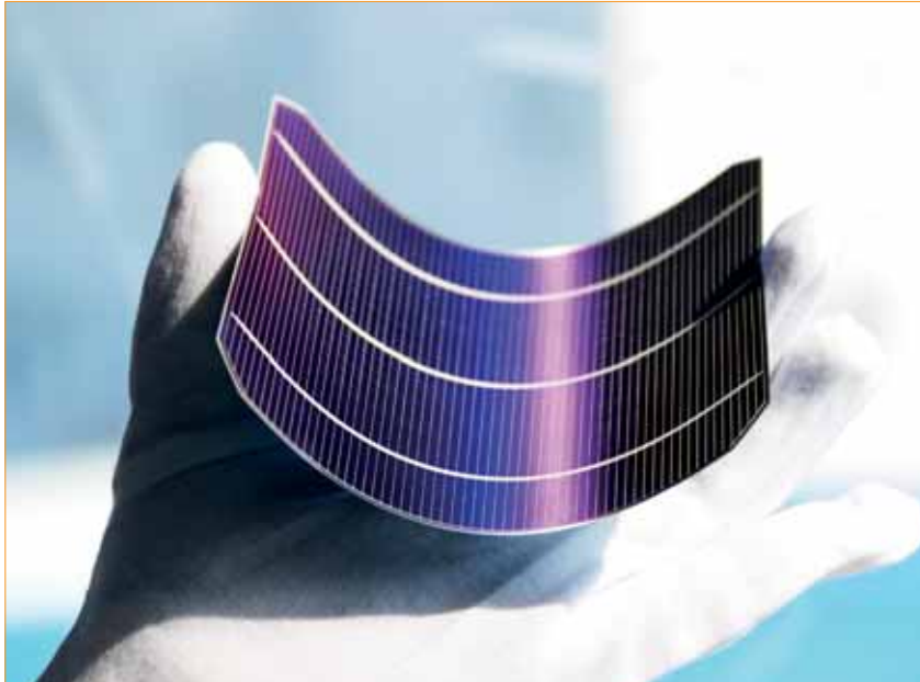
Figure 5. A flexible solar cell made from a LONGi 100 \mu m wafer.
