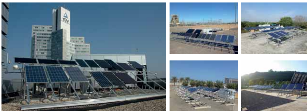
Figure 1. The test sites operated by TÜV Rheinland for PV module characterization and energy yield measurements (clockwise from left): Cologne (Germany, moderate climate), Tempe (Arizona, dry continental climate), Chennai (India, tropic climate), Thuwal (Saudi Arabia, dry desert climate with sand deposition) and Ancona (Italy, Mediterranean climate).
