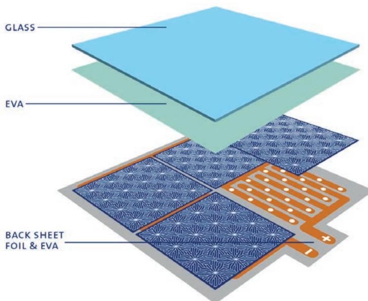
Figure 1. Schematic expanded view of the integrated backsheet approach.
