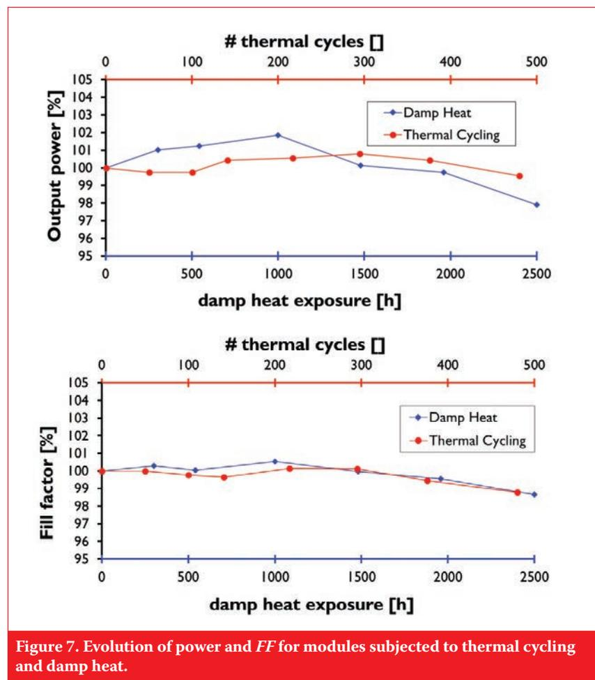
Figure 7. Evolution of power and FF for modules subjected to thermal cycling and damp heat.
