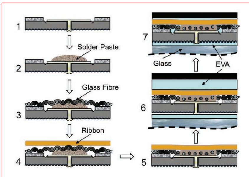
Figure 2. Schematic overview of the process flow.
