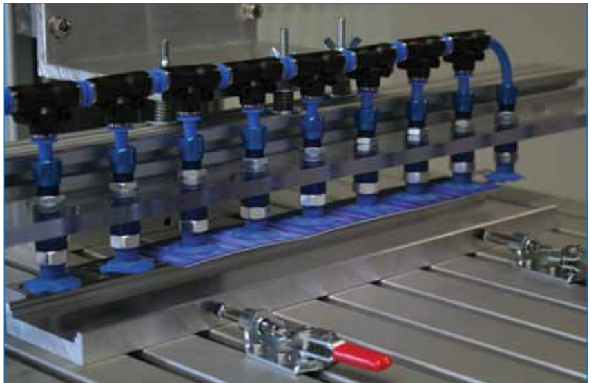
Figure 10. Photograph of assisted string handling during receiver production.
