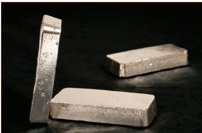
Figure 2. Silver's unique properties as a highly conductive metal that forms stable connections to crystalline silicon means it is very hard to replace with another single material.
