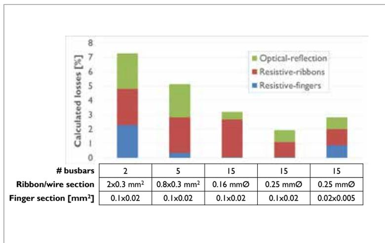
**Figure 4. The relative impact of amount and cross-section of ribbons/wires, and cross-section of fingers in (calculated) resistive and optical losses due to interconnection (illustrative numbers, assuming fixed amount of fingers and finger and ribbon conductivity).**
