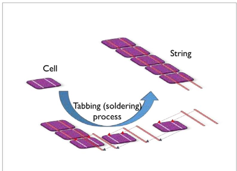
Figure 3. Standard interconnection of two-side-contacted cells into strings is achieved through alternately laying down and soldering of cells and ribbons in the so-called tabbing process.
