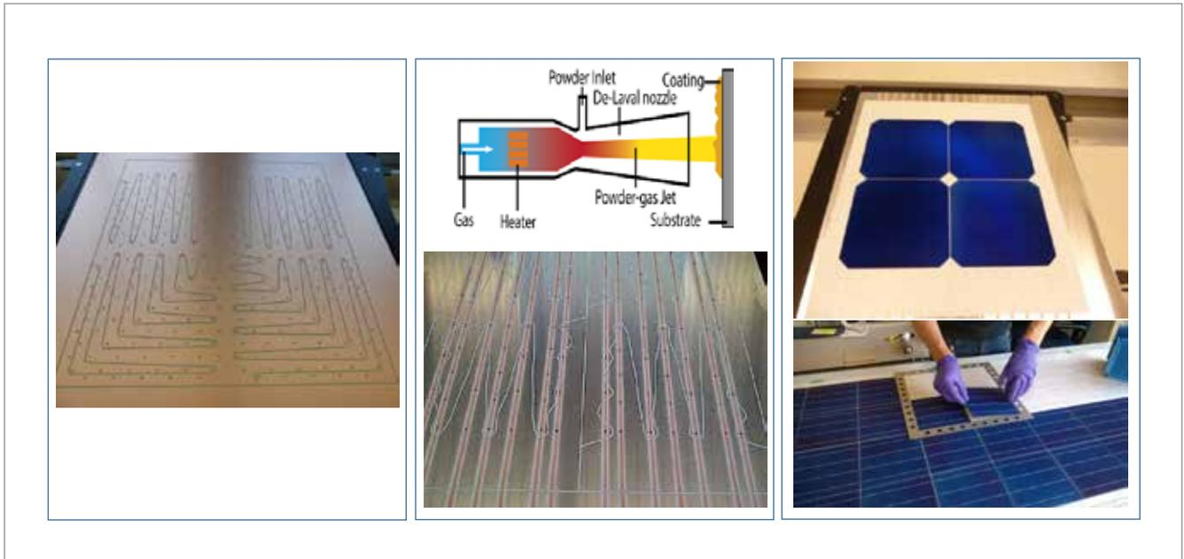
**Figure 12. From left to right: a patterned copper conductive backsheet (left), a schematic representation of the spray gun used for the cold spray process and an aluminium foil with sprayed copper lines corresponding with the position of positive and negative contacts (middle); an IBC 2x2 cells mini module and the manufacturing of a MWT full size module based on copper sprayed aluminium conductive back sheets.**
