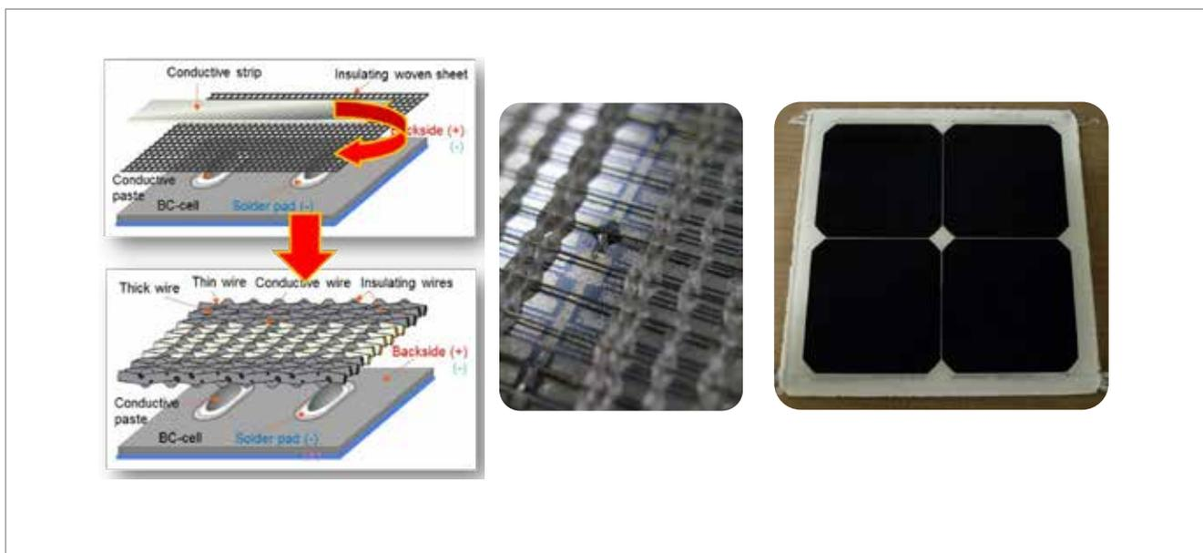
**Figure 14.** Schematic (left) and detail (middle) of how the interconnecting conductive ribbons in the solder-through approach can be integrated inside the woven fabric and applied in a 2x2-cell-module (right).
