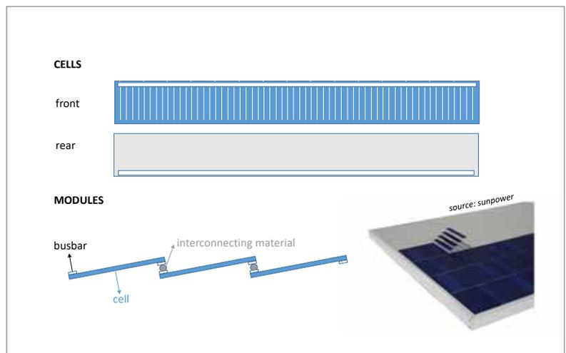
**Figure 8. Schematic layout showing the principle of shingling module technology: above a top view of a monofacial sliced cell with busbars at the leading edges of front and rear cells; lower left a cross section of the interconnection of the sliced cells via an interconnecting material and lower right how cells are integrated in a full size module. Source: SunPower.**
