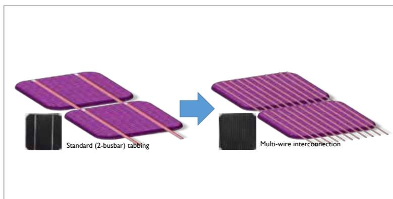
**Figure 5. Illustrating the evolution in appearance (small insets) and interconnection scheme from standard (two-busbar) tabbing (left) to multi-wire interconnection (right).**
