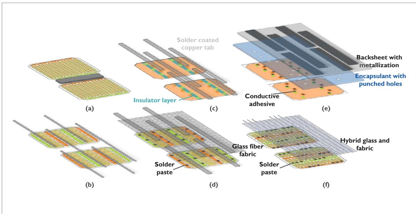
**Figure 9. Schematics of various interconnection approaches for back-contact cells: (a) edge stringing, (b) busbar soldering (c) point soldering, (d) solder-through stringing, (e) foil-based interconnection and (f) woven multi-wire interconnection fabric (figure reproduced from [25] with permission).**
