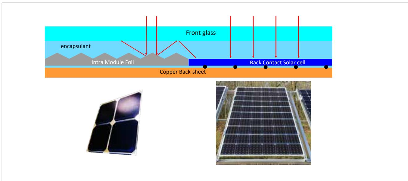
**Figure 13.** Upper: schematic cross-section of a Foil-based back contact module combined with reflective Intra-Module Foil (IMF). Lower left: IBC mini-module with 8mm wide IMF integrated along cell edges and corners, lower right: full size 60-cell MWT module using IMF materials to increase the current by almost 6%.
