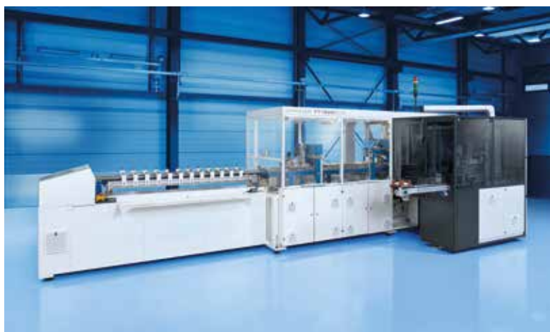
Figure 7. The TT1600 ECA solar cell stringer from the Germany-based company teamtechnik, capable of producing glued HJT strings at a throughput of 2.3 sec per cell and 1,600 cells per hour.
