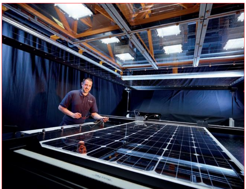
Figure 3. TÜV Rheinland steady-state solar simulator.
