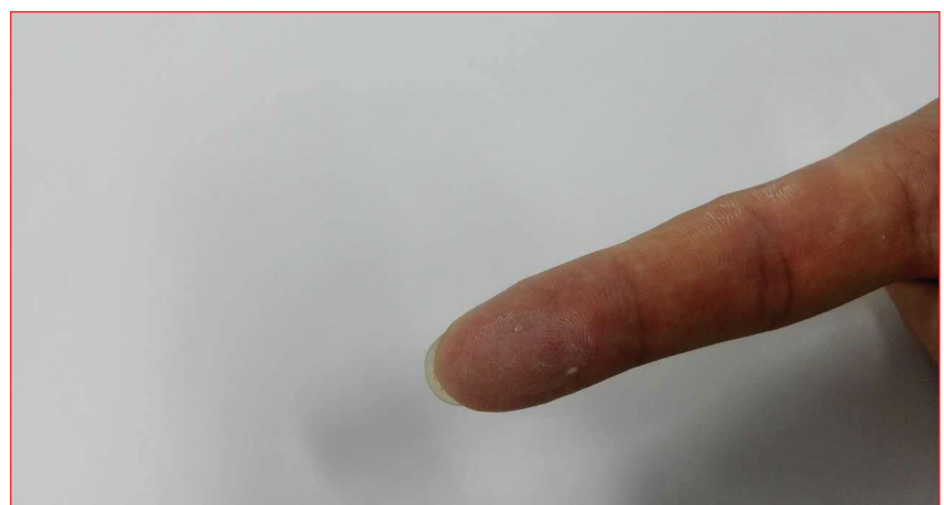
Figure 6. White powder from the Tedlar surface, observed after 330kWh/m 2 of UV exposure.
