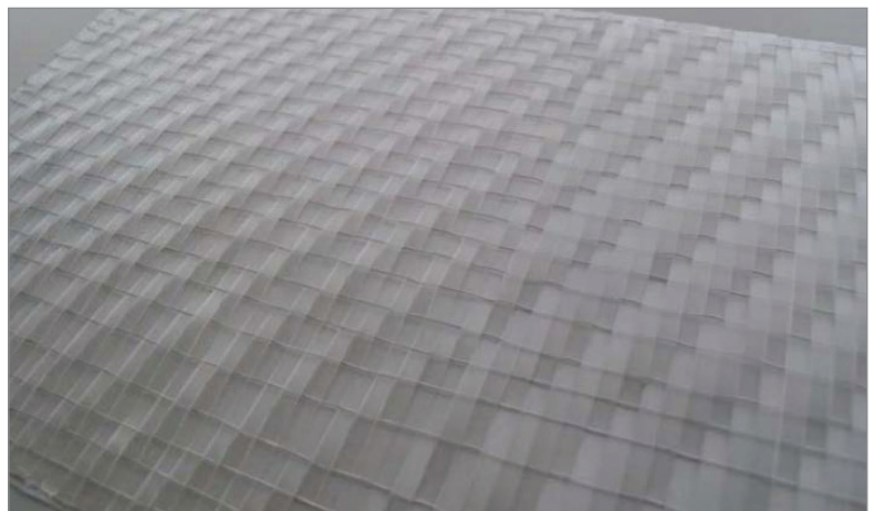
Figure 9. Example of a woven interconnection sheet.
