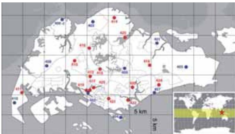
Figure 3. A network of 25 ground-based irradiance measurement stations in Singapore. The blue dots represent stations where both silicon reference cells and pyranometers are deployed. The red dots are stations where only reference cells are installed. The bottom right corner shows Singapore's position (red star) on the world map, as well as the 'sunbelt' region (yellow band) between the tropics of Cancer and Capricorn.
