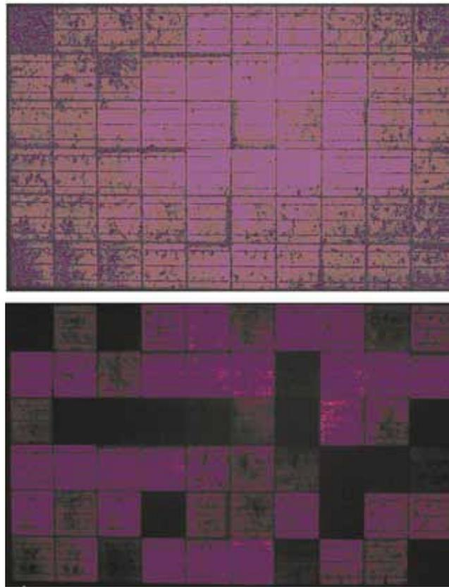
Figure 9. Results of an accelerated PID test (48h at -1000V) in a climate chamber (damp heat: 85°C, 85% r.h.). Top: module in initial state. Bottom: same module after treatment, with a loss of 40% of initial STC power output.
