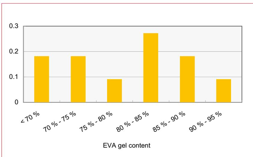
Figure 7. Frequency distribution of EVA gel content of analyzed solar modules from manufacturer A.
