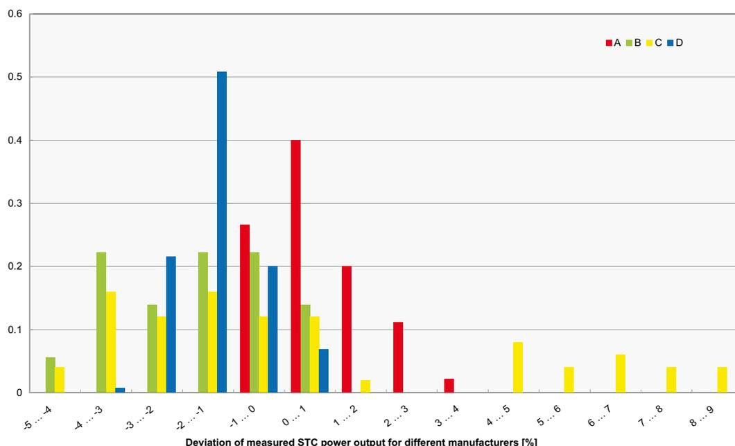
Figure 4. Frequency distribution of deviations of the independently measured STC power output from the labelled power for modules from four different manufacturers A, B, C and D.
