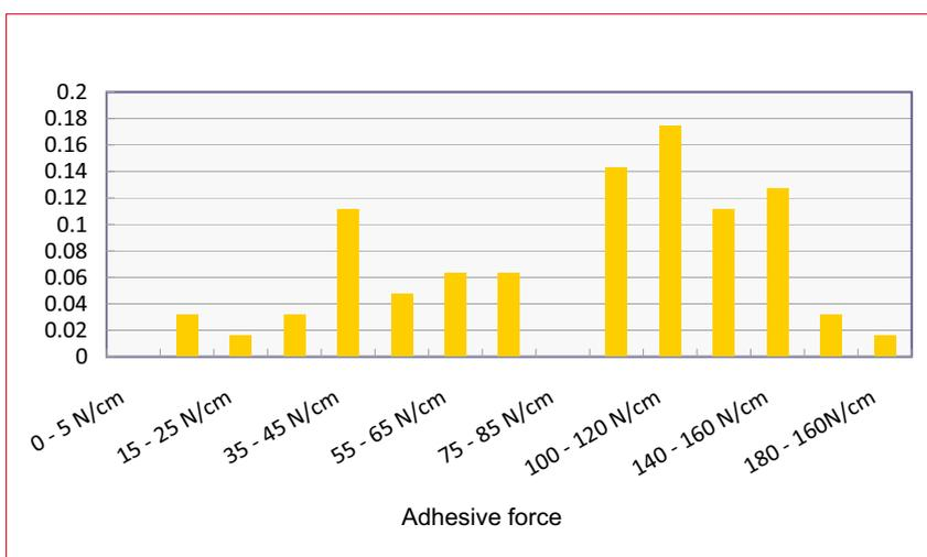
Figure 8. Frequency distribution of the measured adhesive force between EVA and glass.
