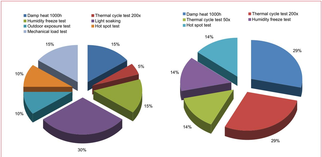
Figure 2. Comparison of failures during the certification processes for thin-film technology modules (left) and c-Si technology modules (right).
