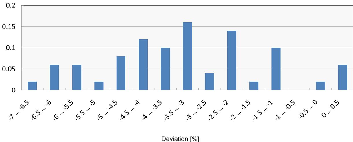
Figure 12. Deviation of measured and labelled STC power output of separate strings of modules in operating photovoltaic systems.
