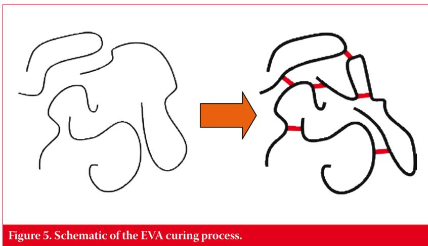
Figure 5. Schematic of the EVA curing process.
