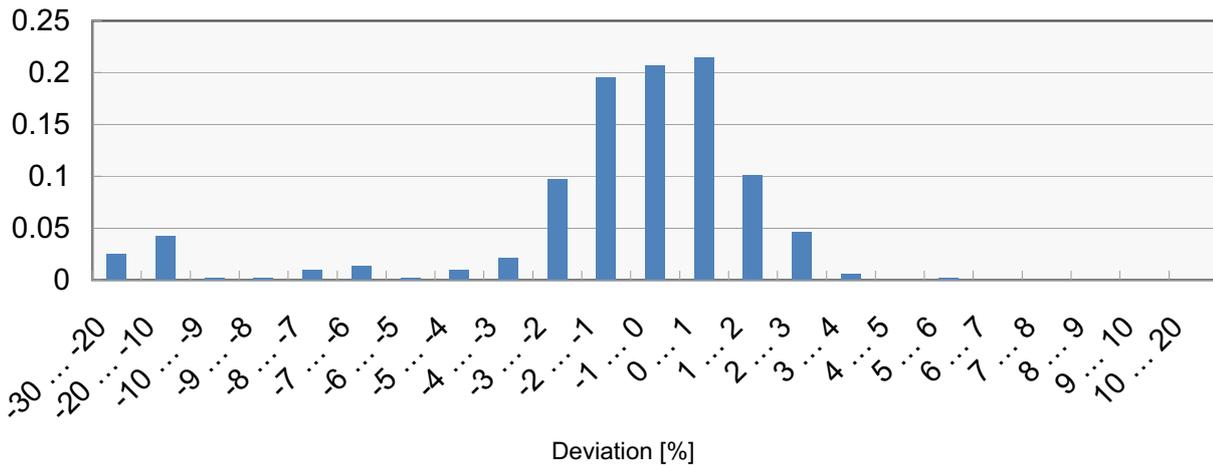
Figure 11. Deviation between measured and labelled STC power output of unmounted photovoltaic system modules.
