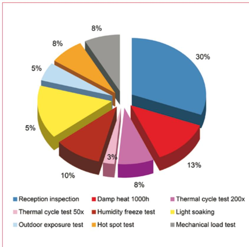
Figure 1. Distribution of fail criteria during the certification process for all tested modules.
