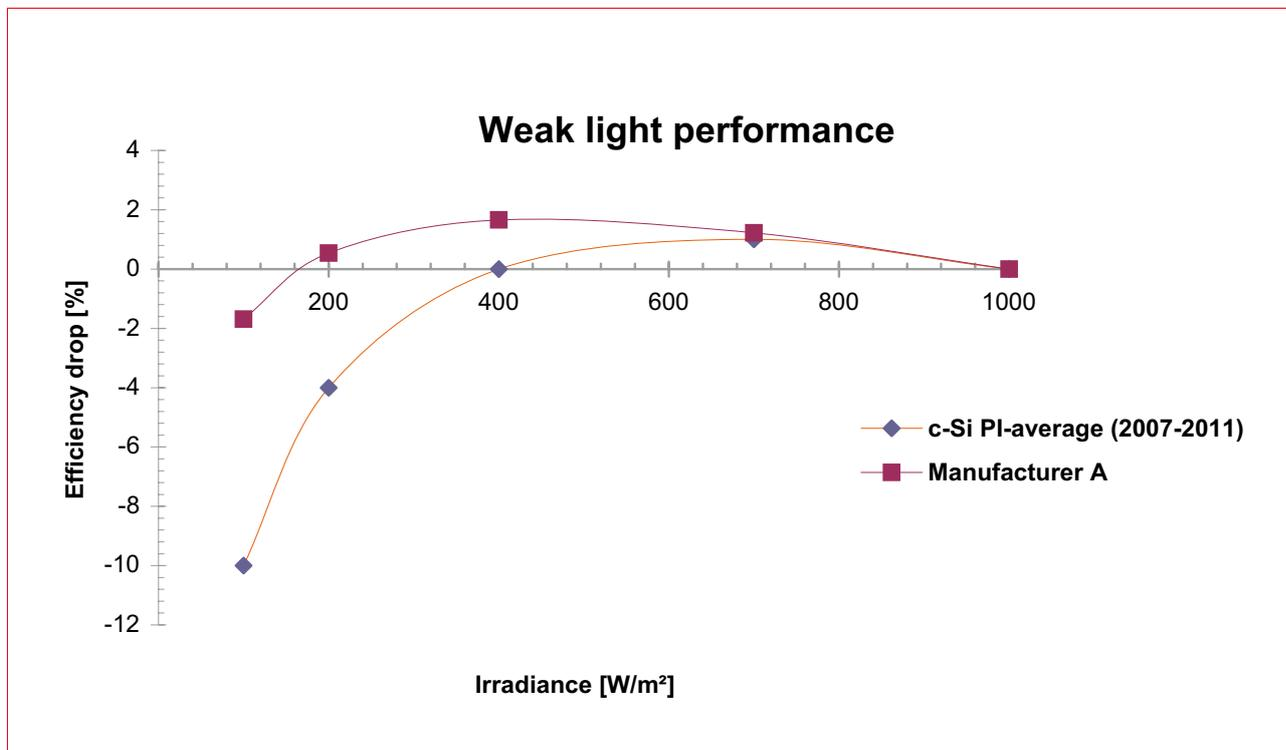
Figure 10. Weak light performance curve of a module with a ‘positive’ weak light behaviour. An efficiency drop of 30% is also possible.
