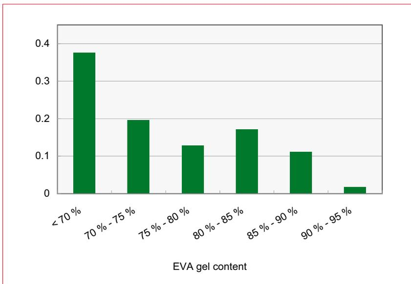
Figure 6. Frequency distribution of EVA gel content of 120 analyzed PV modules.
