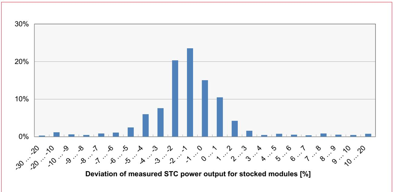
Figure 3. Frequency distribution of deviations of the independently measured STC power output from the labelled power for ex stock modules.
