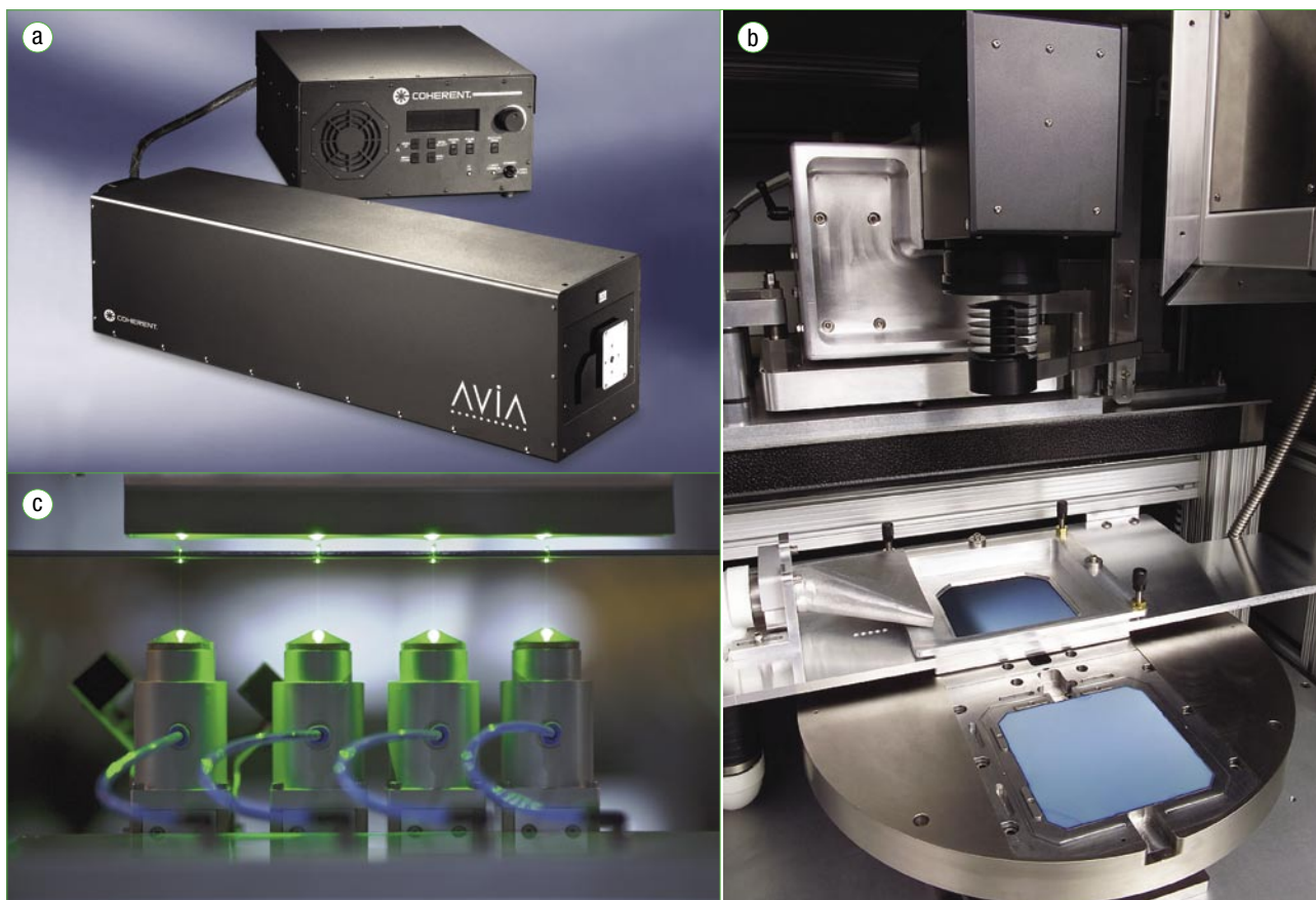
Figure 1. A laser-based tool is typically comprised of a laser source (a), like the Coherent AVIA. (b) shows a c-Si beam-delivery assembly taking the laser beam from source to sample; scanner (black box, top centre), c-Si vacuum chuck and wafer turntable. In thin-film tools, beams can be split for simultaneous patterning (c), courtesy of Oerlikon Solar Ltd., Trübbach, Switzerland.
