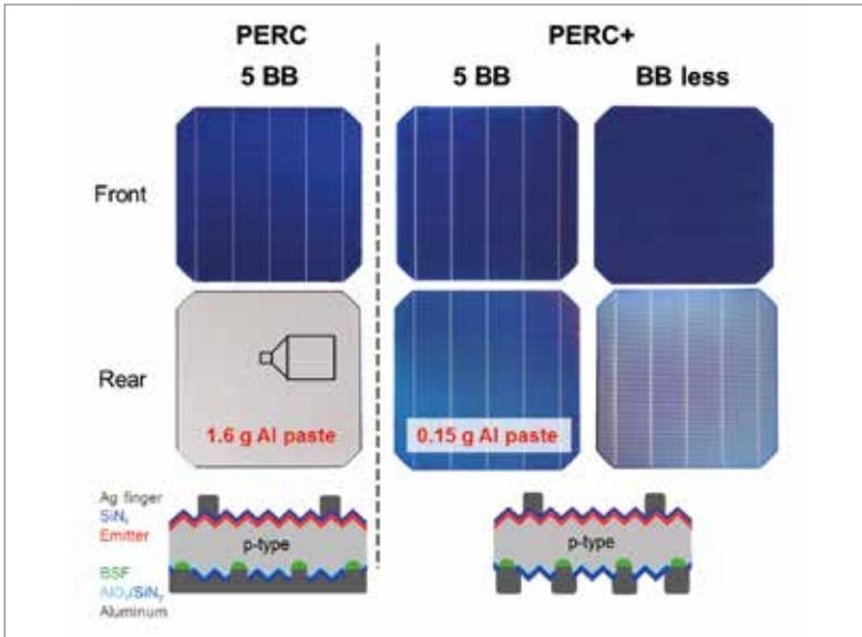
**Figure 1. Photographs of the front and rear sides, as well as schematic cross-section drawings, of industrial PERC and PERC+ solar cells. PERC+ cells enable bifacial application and reduce the Al paste consumption, while using the same processing sequence as industrial PERC solar cells.**
