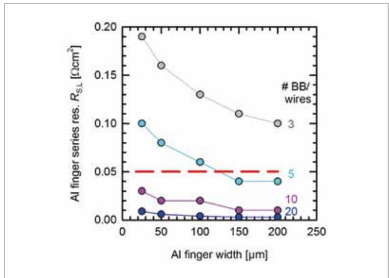
**Figure 2. Calculated series resistance contribution  $R_{sL}$  of the Al finger grid as a function of the number of busbars/wires and the Al finger width.**
