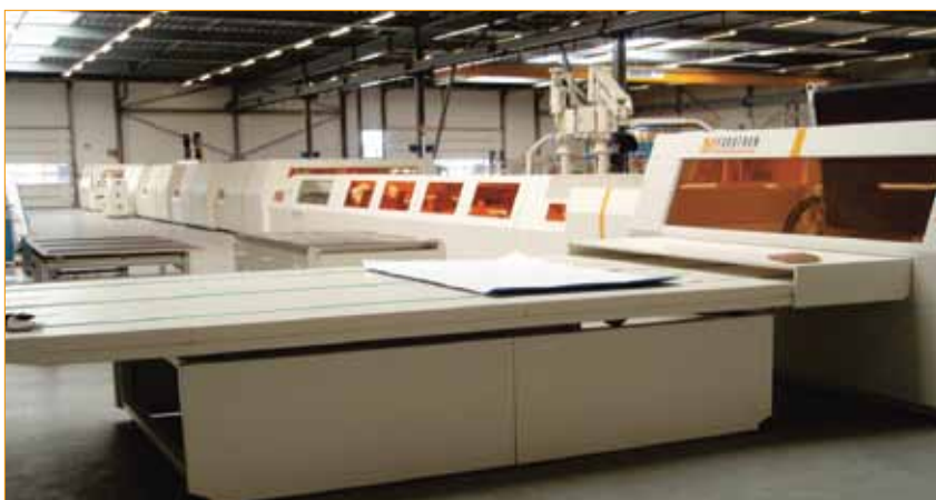
Figure 2. Assembly line for the MWT modules used in the experiments.
