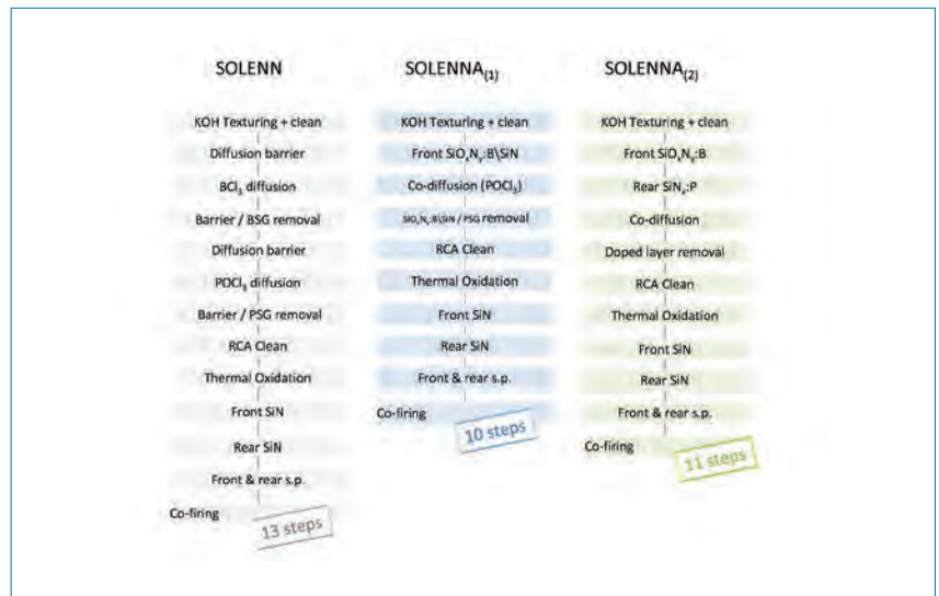
Figure 3. The n-PERT process flow simplifications: gaseous diffusion route (SOLENN), co-diffusion SiO x N y :B/POCl 3 route (SOLENNA (1) ) and full dielectric co-diffusion route (SOLENNA (2) ).
