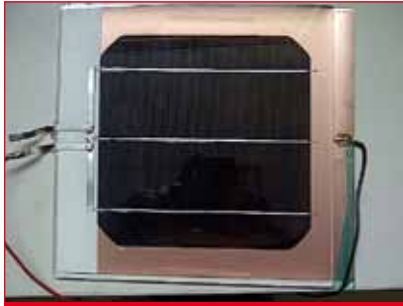
Figure 7. Image of a pseudo-MWT mini-module. The front-side interconnection is accomplished by soldering tabs to the busbars; the rear contact to a conductive backsheets is made by a conductive adhesive printed at the location of the busbars on the rear of the cell.
