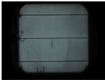
Figure 10. EL image of a single-cell module after 100 thermal cycles, showing little change relative to the module at t = 0 . The module shows uniform illumination, indicating that the cell and interconnections are intact.
