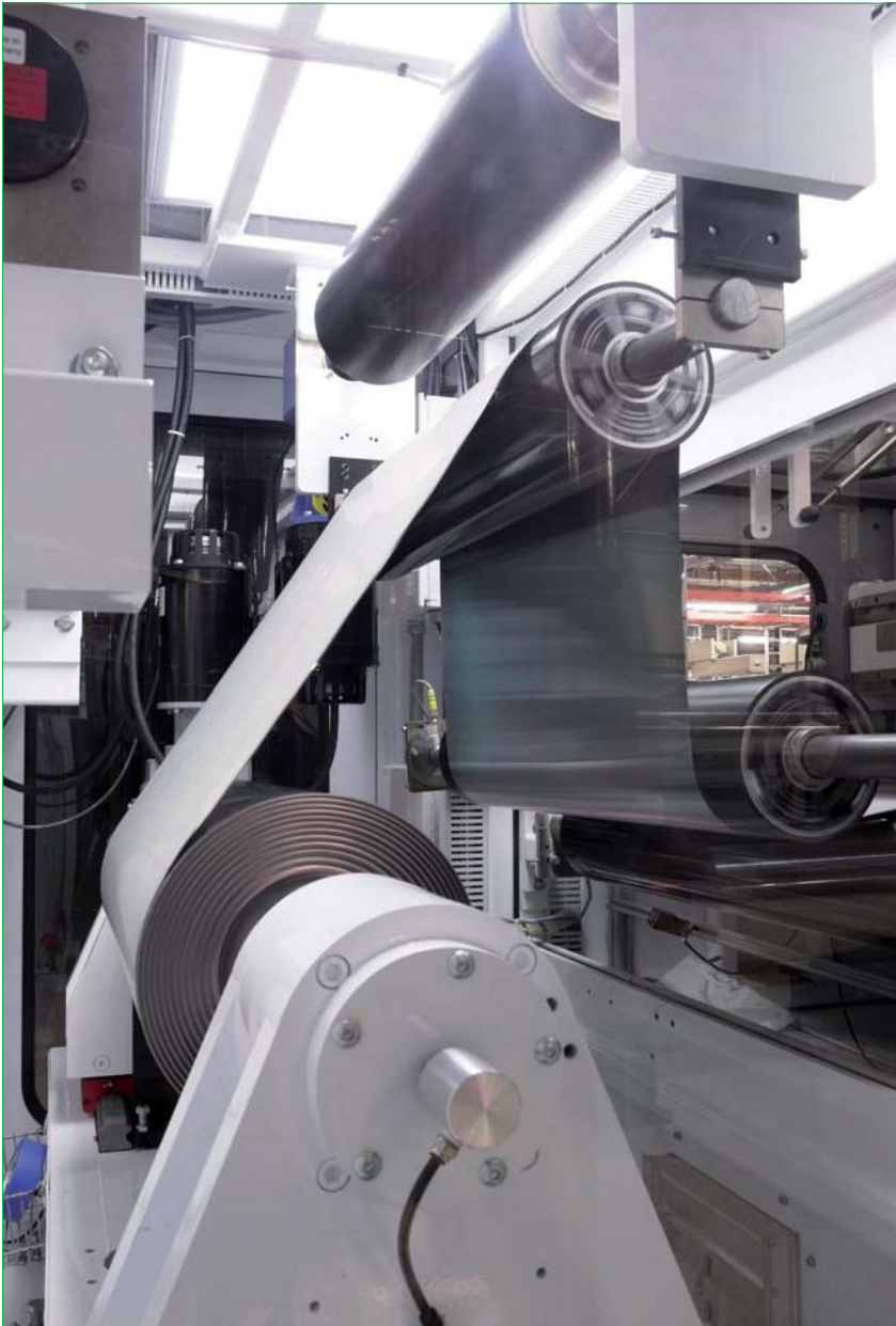
Nanosolar uses a proprietary ink-based process on its roll-to-roll CIGS solar-cell production line.
