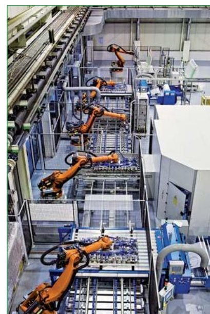
Nanosolar's fully automated panel assembly factory is rated at an annual capacity of 640MW.
