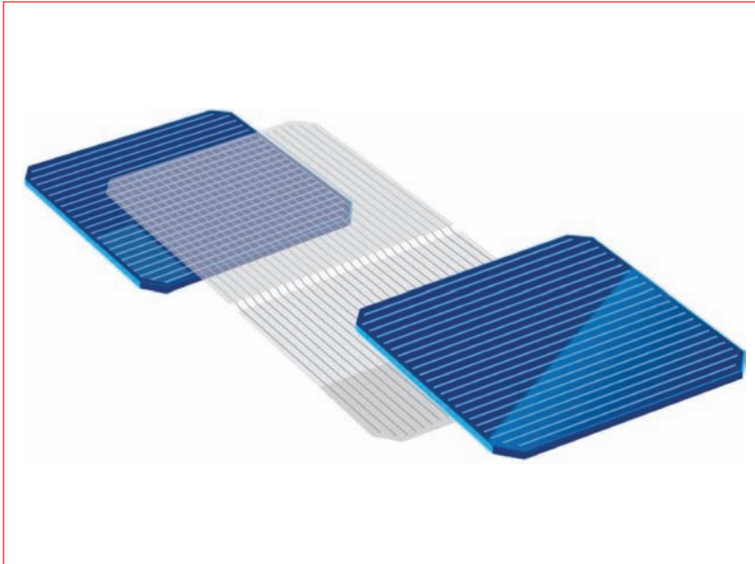
Figure 3. Schematic representation of SmartWire technology, showing the metal fingers of a single cell contacted with smart wires.
