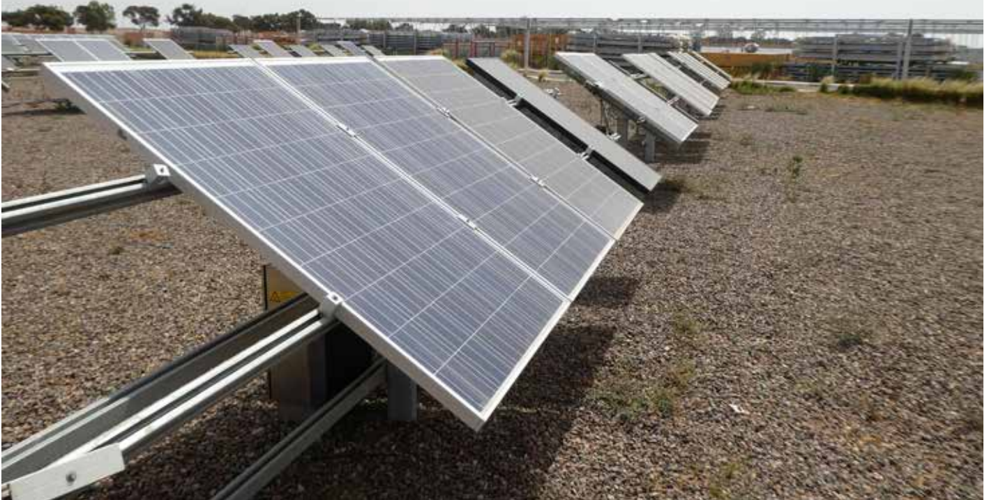
Picture 1. Outdoor measuring set-up and installed PV modules in Green Energy Park of IRESEN, Ben Guerir, Morocco [8]
