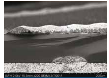
Figure 6. SEM cross-section image of a screen-printed, rear-side-passivated PERC solar cell with local line contacts on the rear side. Horizontal dimensions of the finger width and the line contact width deduced from this image have to be divided by \sqrt{2} , due to the 45-degree cross-section angle.
