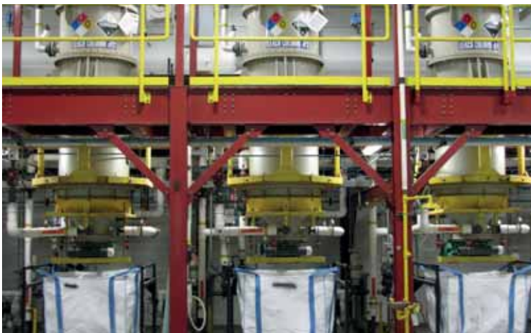
Figure 6. First Solar's second-generation recycling technology based on the chemical industry's batch process.
