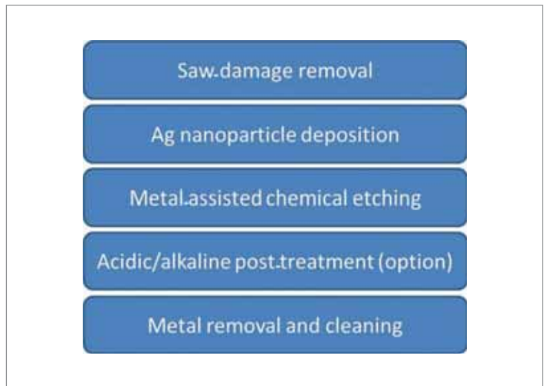
Figure 4. Generic process flow for black silicon based on metal catalyst chemical etching (MCCE) [9].
