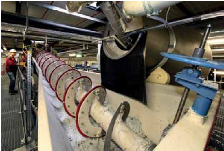
Figure 5. First Solar's first-generation recycling technology based on the mining industry's batch process.
