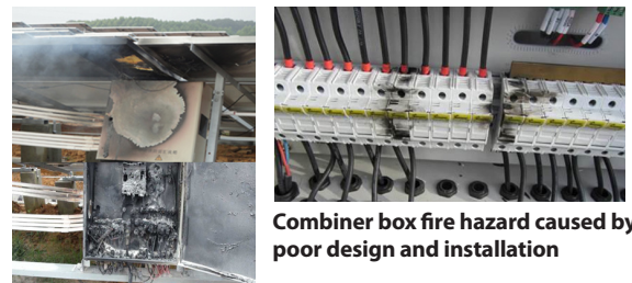
IGBT inverter explosion/fire hazard caused by poor inverter quality and technical design.
