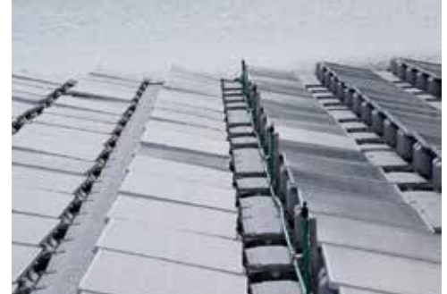
Figure 9. Sunseap/C&T testbed system with active cooling
