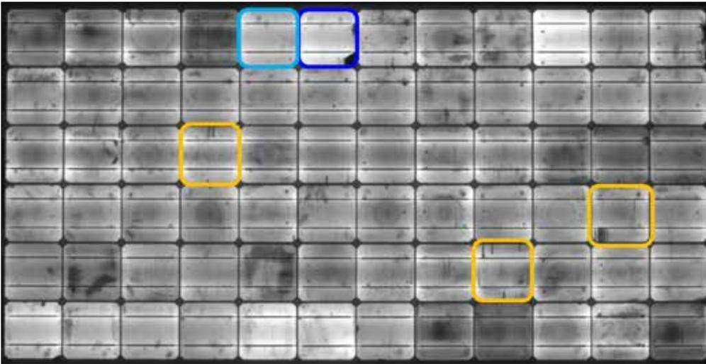
**Figure 5. Sample of a poor module from the field after five years of operation: cell mismatch, micro cracks (light-blue), isolated cell area (blue) and finger interruptions (yellow), power loss: -5% in relation to data sheet (0 ...+3%)**
