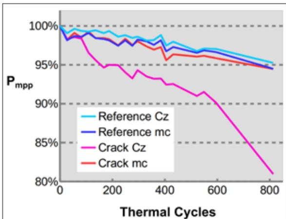
**Figure 7. Degradation of test modules during extended thermal cycling testing. Reference samples without cell micro cracks (blue/cyan) show linear degradation of 0.5% per 100 TC. A mc module having a medium-sized cell micro crack (red) shows the same result, whereas a Cz module with a long micro crack (magenta) shows much stronger degradation**
