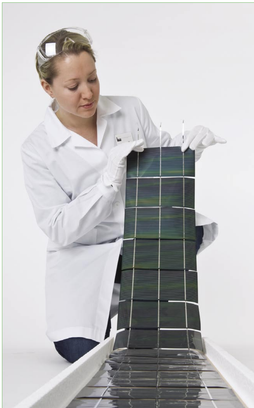
Figure 6. Global's PowerFlex strings can be integrated into standard modules.
