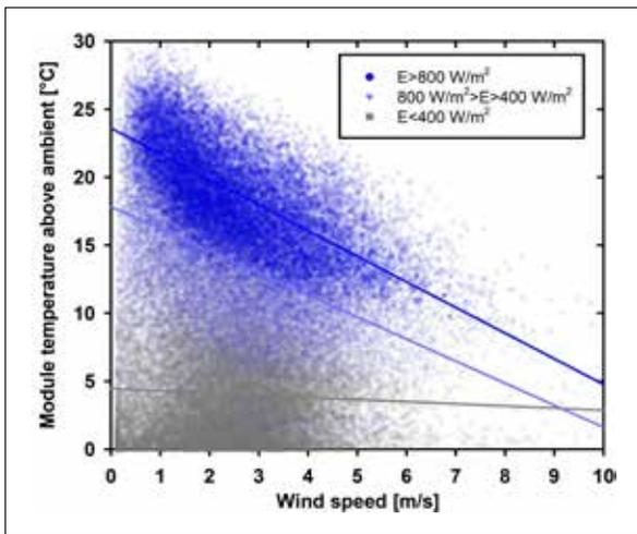
**Figure 7. Impact of wind speed on (tracker) module temperature for three irradiance levels (five-minute mean values)**
