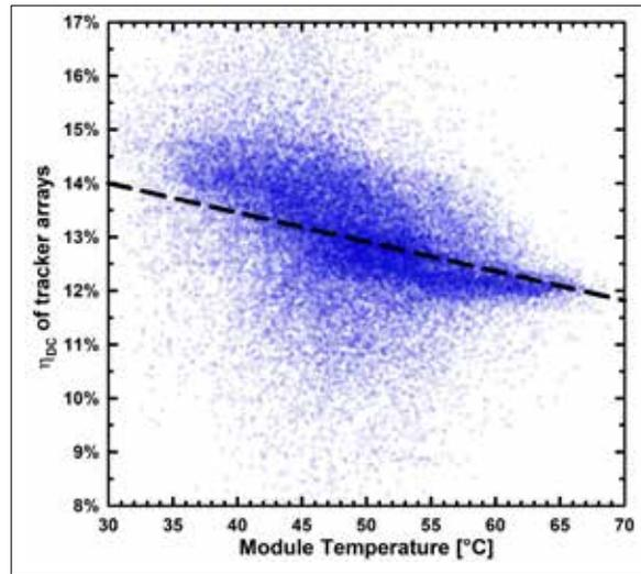
**Figure 6. Array DC efficiency as a function of temperature (five-minute intervals,  $E > 400\text{W/m}^2$ ). The line illustrates the power temperature coefficient of  $-0.41\%/^{\circ}\text{C}$  specified for these modules [6]**
