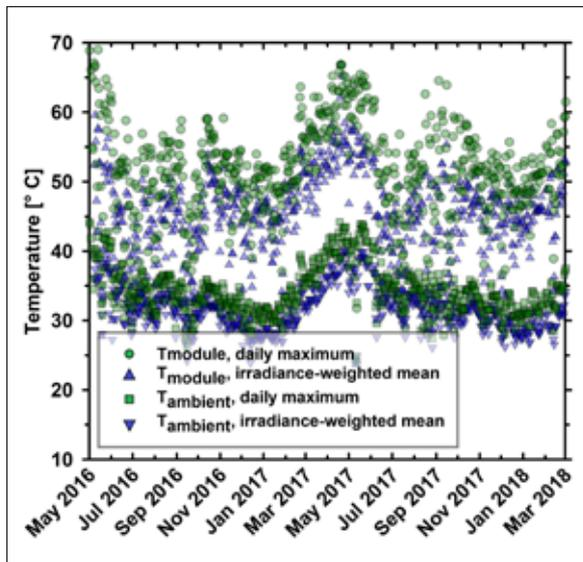
**Figure 5. Daily module and ambient temperatures: maxima and irradiance-weighted means**
