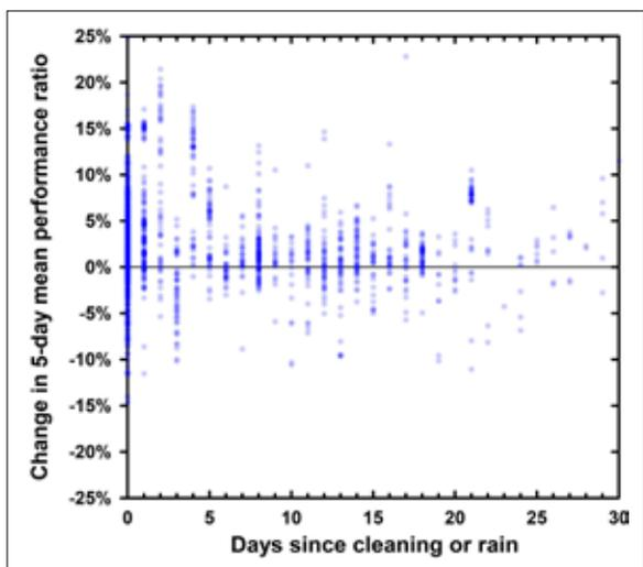
**Figure 8. Relative change in DC performance ratio before and after cleaning and rain events, using a five-day mean**
