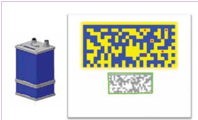
Figure 7. Example of an industrial type data-matrix reader from IOSS GmbH (left). This reader has adjustable light and camera parameters in order to optimize readability, which is indicated by the red dots in the right-hand image.
