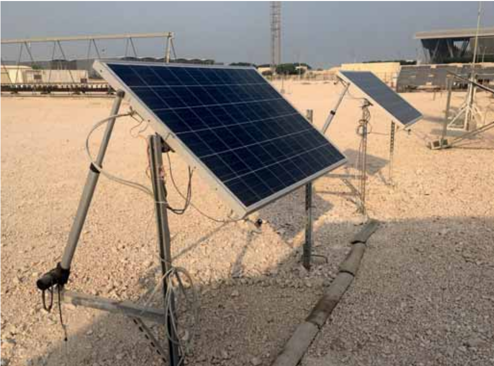
Figure 7. Test trackers with enhanced tilt ranges at the OTF in Qatar. Soiling was greatly reduced by vertical night stowing, but there was little gain from tilting to enhance dust resuspension during wind [13]
