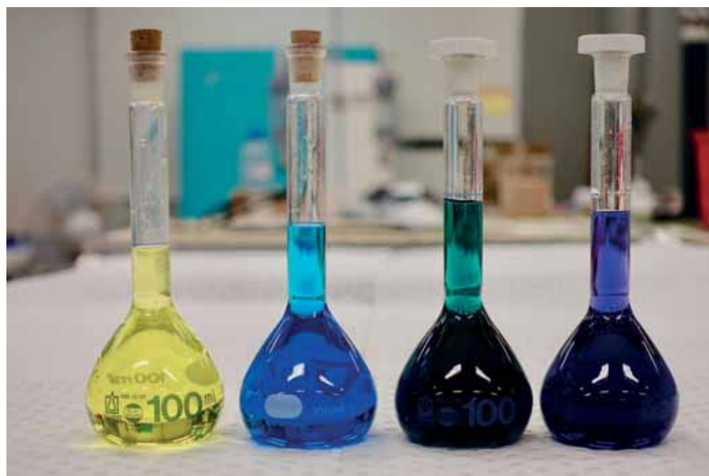
Colours of different oxidation states of vanadium from left to right: \text{VO}_2^+ , \text{VO}^{2+} , \text{V}^{3+} , \text{V}^{2+}
