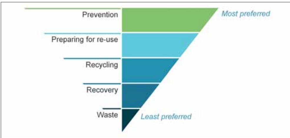
Figure 3. Waste hierarchy, also applicable to PV EoL management, according to the EU waste legislation
