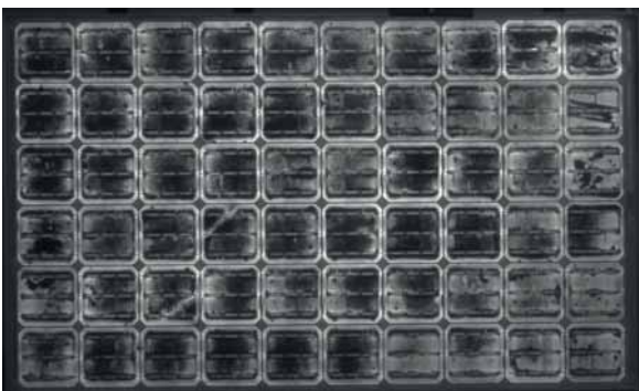
Figure 10. Module after installation on Island A for six years
