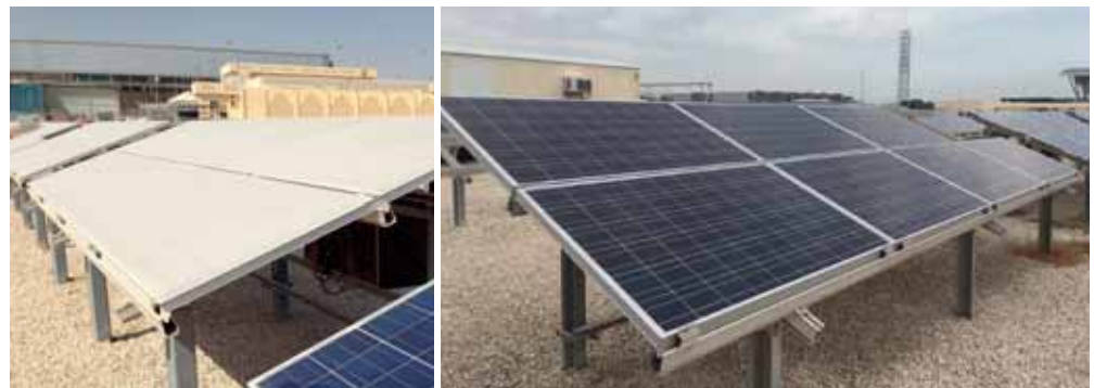
Figure 1. Examples of soiled modules (left) and modules naturally cleaned by heavy rain (right). These are the same test beds viewed from opposite side at the QEERI Outdoor Test Facility
