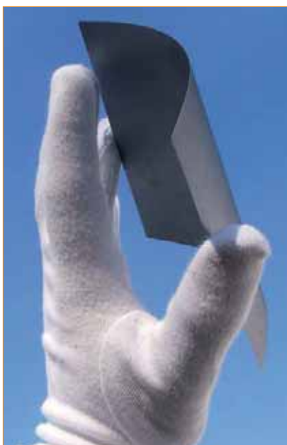
Figure 8. Photo of a 70µm multi-crystalline wafer, which demonstrates the flexibility of thin wafers.
