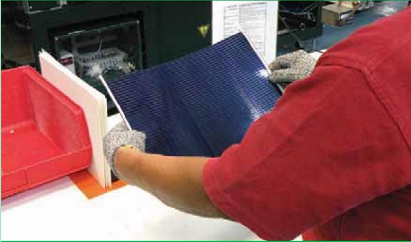
Uni-Solar's triple-junction amorphous-silicon thin-film PV laminates.
