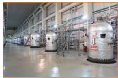
Polysilicon reactors at LDK Solar's Ma Hong polysilicon plant.
