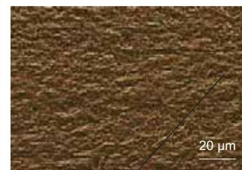
Figure 3. SEM micrograph of a typical surface of an as-sawn multicrystalline silicon wafer.
