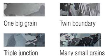
**Figure 1. Four of the groups of specimens showing different crystallinity features.**
