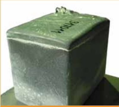
Figure 8. Example of a small ingot casted by SolarWorld AG for the SolarFocus project in 2008, similar to the ingots of the materials B1 and B2 in Fig. 7.
