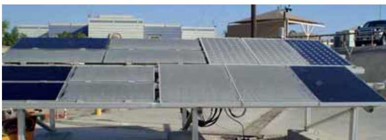
◀ Figure 2. Test field in Dhahran, Saudi Arabia (photo taken on 1 November 2010 after partial cleaning).
