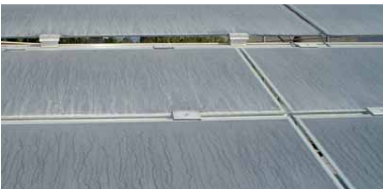
◀ Figure 3. Zoom-in on the polluted modules of the test field.
