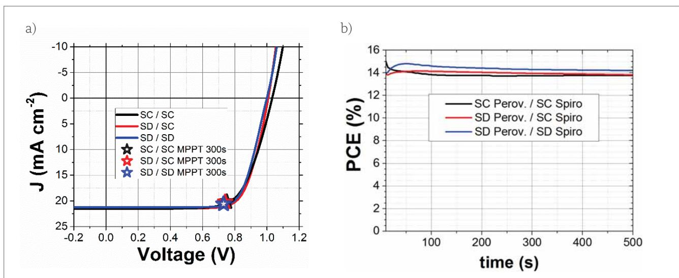
**Figure 5. Illustration of the feasibility of replacing spin coating (SC) by scalable slot die (SD) coating technology in perovskite cell processing: (a) typical  $J$ - $V$  curve of the perovskite cells; (b) typical maximum-power-point tracking (MPPT) curves for the devices, measured under maximum-power-point voltage bias, from Di Giacomo et al. [17]. (Perov. = perovskite absorber layer; Spiro = spiro-OMeTAD charge contact layer.) Reprinted with permission from Di Giacomo et al. [17].**
