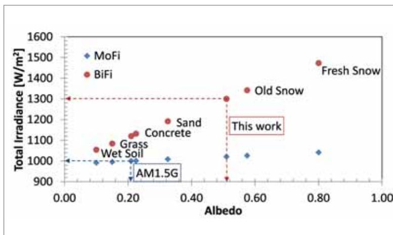
Figure 4. Analysis of the albedo sensitivity of total irradiance received by bifacial and monofacial PV modules. The simulation was carried out using the environmental conditions as defined in IEC 60904-3.
