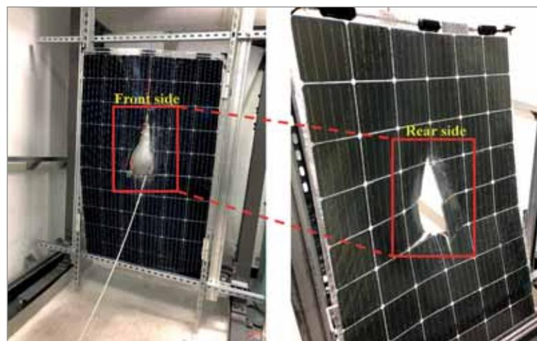
Figure 6. Examples of module breakage test failures of bifacial PV modules observed at the TÜV Rheinland laboratory.
