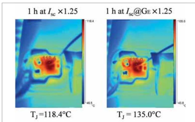
Figure 5. Example of elevated diode junction temperature observed by the TÜV Rheinland laboratory during the bypass diode thermal test with enhanced test current.
