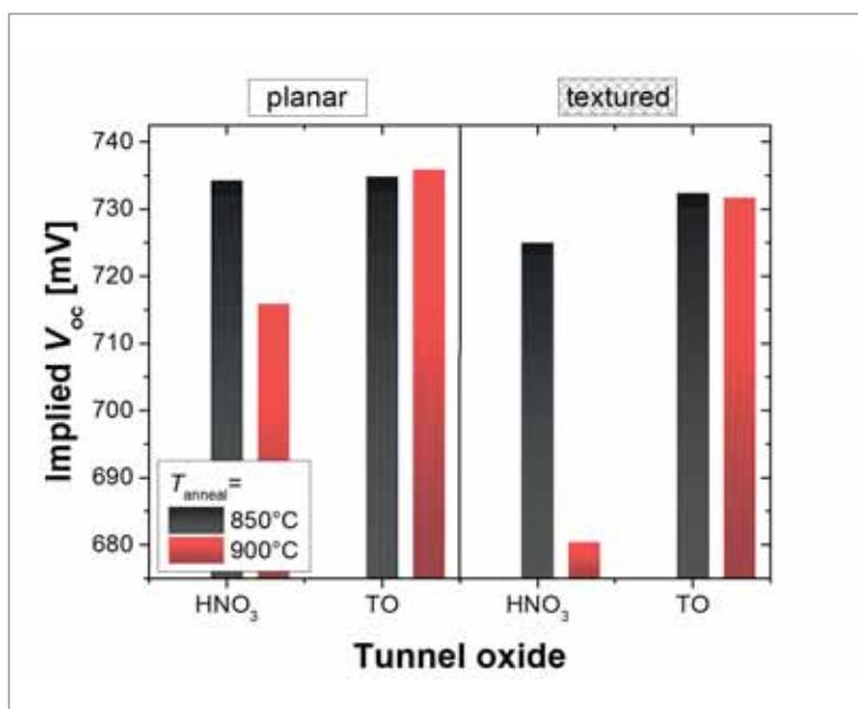
Figure 4. *iV<sub>oc</sub>* achieved by n-TOPCon on planar and textured surfaces respectively. Two different interfacial oxides are compared.
