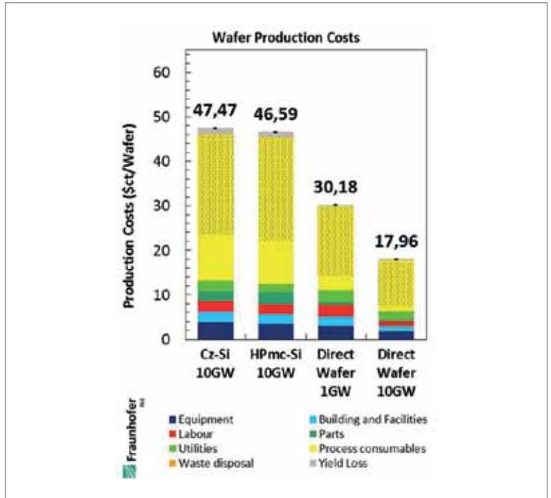
Figure 3. Results of the economic assessment of ingot and wafer production for Cz-Si and HP mc-Si wafers, and of the innovative Direct Wafer approaches (the poly-Si share of process consumables is indicated by the shaded area).
