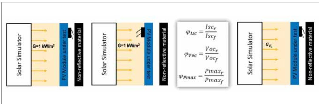
Figure 2. Schematic of the single-side illumination test method for bifacial PV modules.
