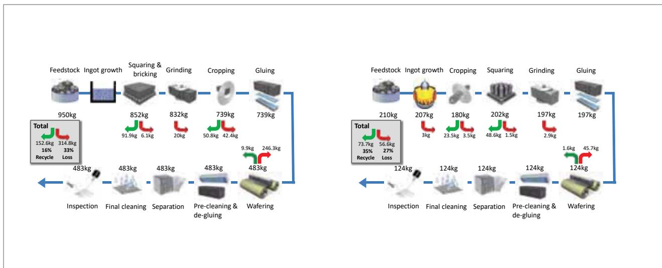
technique has been the predominant method for the cutting of monocrystalline silicon for many years, the major shift to DW cutting for multicrystalline silicon only began in 2017, but it has already become the main technique in 2018.
