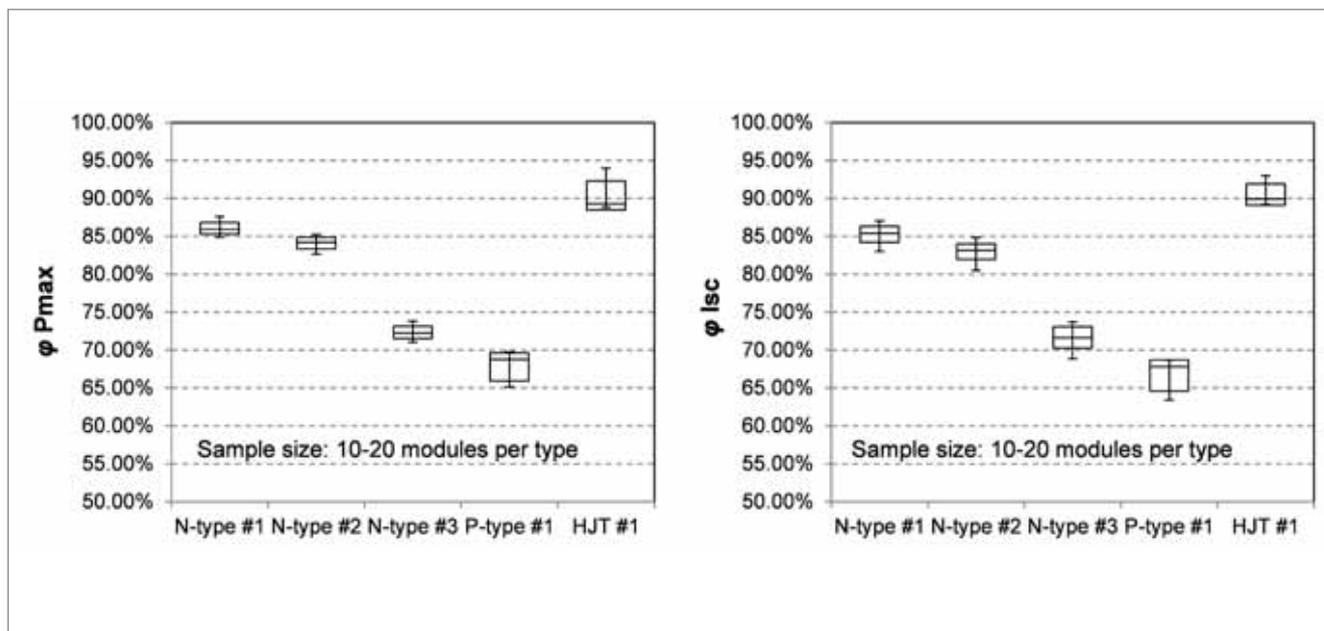
Figure 3. Variations in bifaciality coefficients ( $\phi$ ) of  $P_{max}$  and  $I_{sc}$  evaluated by measuring modules in production from different manufacturers.
