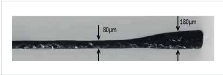
**Figure 12. Example of locally controlled wafer thickness.**
