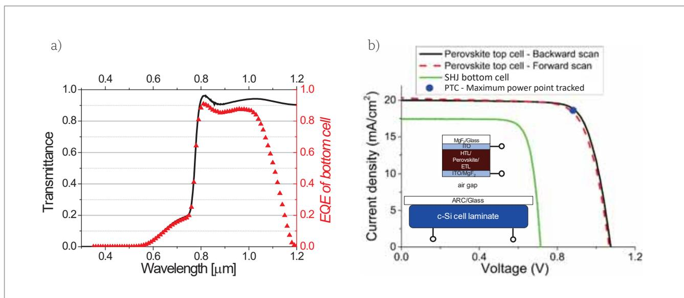
**Figure 3.** Best 4T tandem result obtained at ECN/Solliance: (a) transmittance of the PTC (black), and the filtered EQE of the c-Si SHJ cell (red) [12]; (b) I–V characteristics of the top and bottom cells (the inset shows schematically the configuration of this 4T tandem device).
