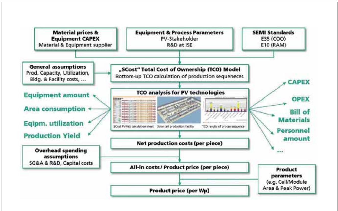
**Figure 2. Methodology for the cost calculation using the SCost tool, developed at Fraunhofer ISE.**
