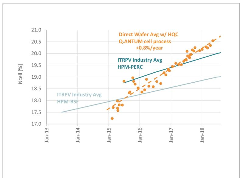
**Figure 10. Evolution of the efficiency gains of Direct Wafer products in combination with Hanwha Q CELLS Q-ANTUM PERC process. Gains exceeding 0.8% per year have consistently been demonstrated.**
