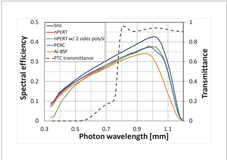
Figure 7. Spectral efficiencies of several types of industrial or industrially processed c-Si cells (solid lines). The transmittance of the perovskite cell stack described in the perovskite/c-Si tandem cell results section is indicated by the dashed line.
