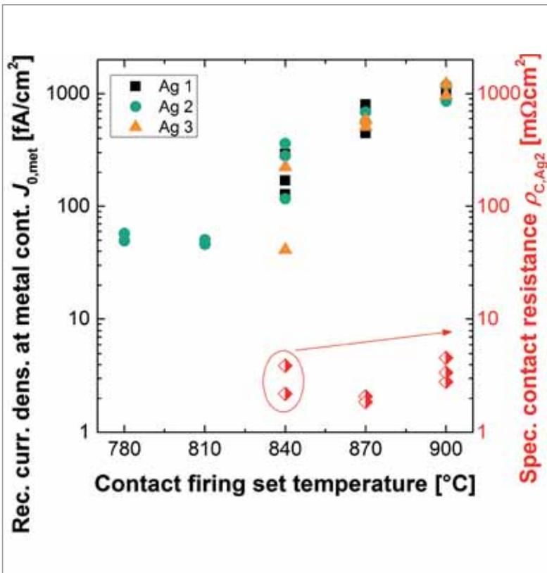
Figure 9.  $J_{0,\text{met}}$  determined by PL imaging at the metallized sites, and  $\rho_c$  of screen-printed silver pastes (Ag 2) on boron-doped poly-Si layers, for different set firing temperatures (Adapted from Mack et al. [20]).
