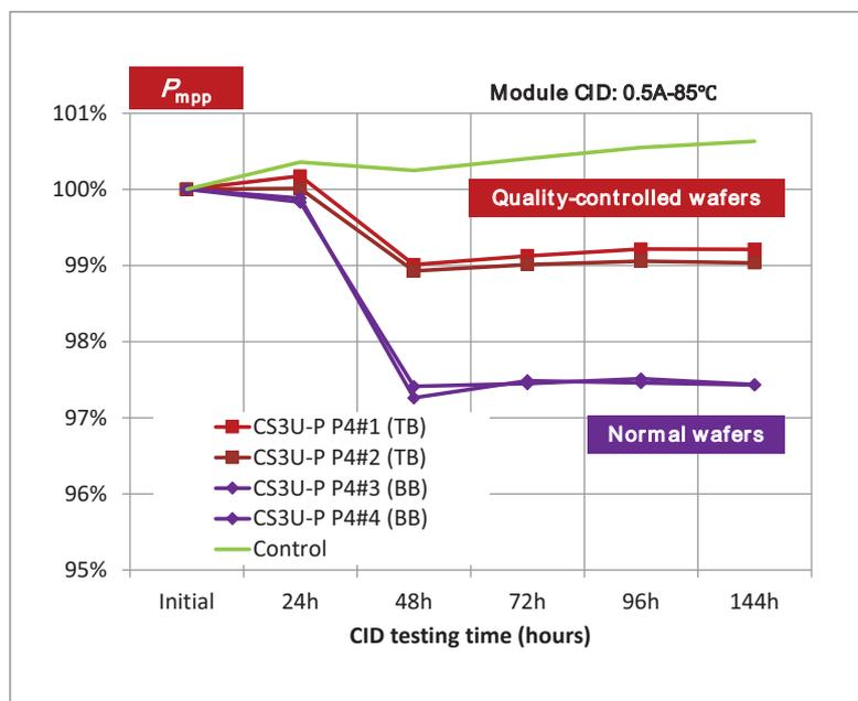
Figure 3. Effect of wafer quality on degradation performance of multi-PERC modules.
