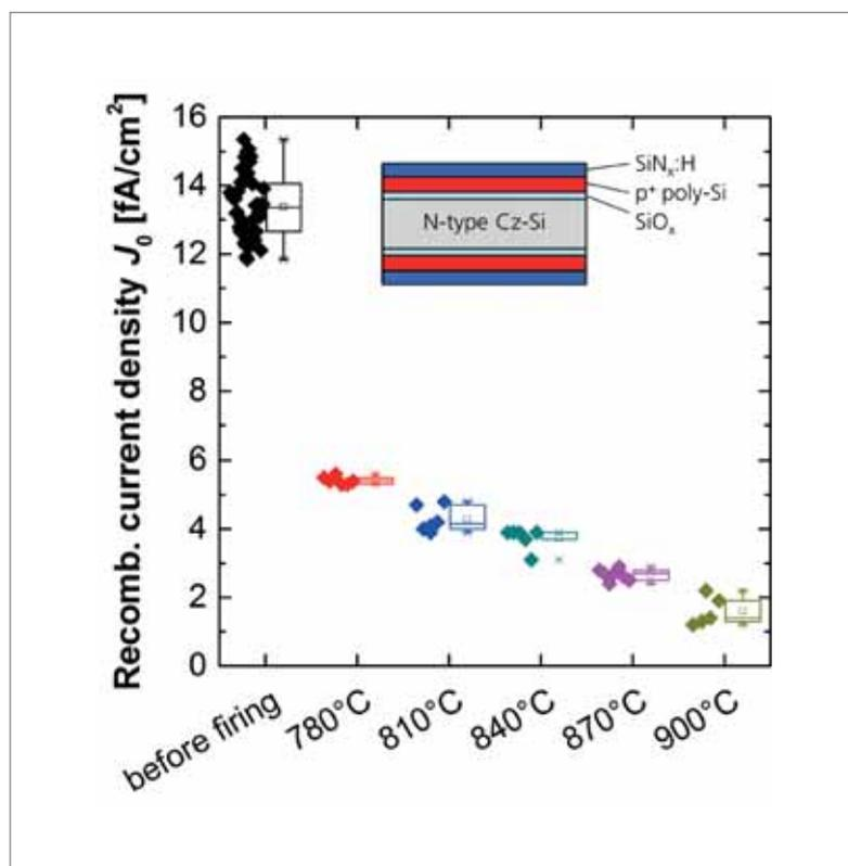
Figure 8.  $J_0$  for each side of symmetrical test structures with interfacial oxide, boron-doped poly-Si layer and  $\text{SiN}_x$  capping, determined after contact firing for different set temperatures [20].
