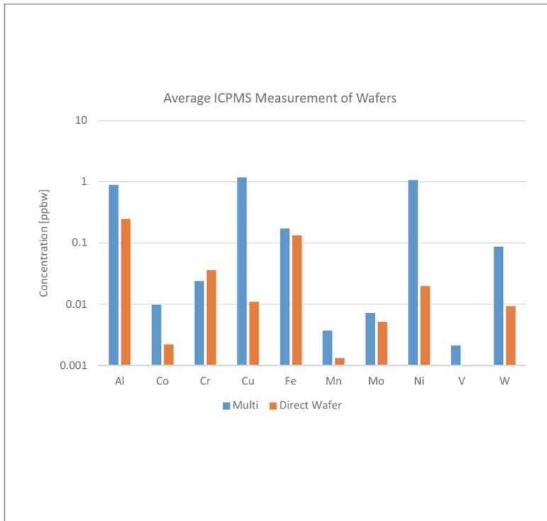
**Figure 8. Comparison of impurity concentrations of wafers produced by mc-Si and Direct Wafer processing. Wacker Chemie AG provided hyperpure polysilicon as raw material, analytical services and technical consulting in the framework of its partnership with 1366 Technologies.**
