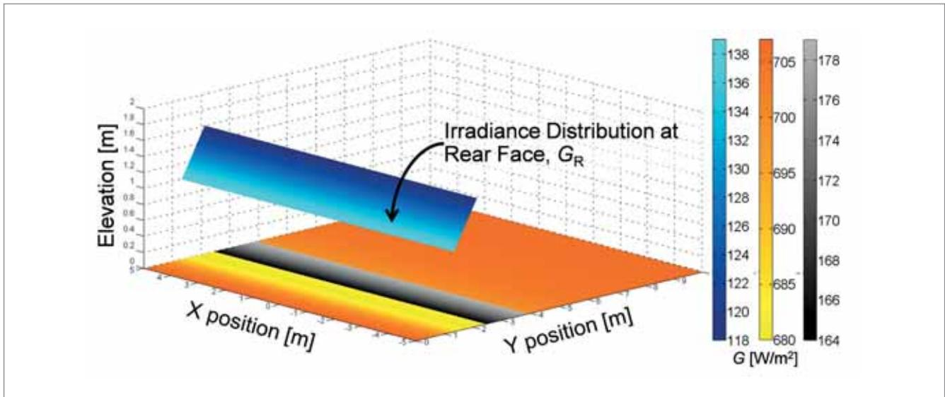
**Figure 1.** Irradiance distribution for a single-row bifacial PV array simulated in the conditions shown in Table 1, without taking into consideration the influence of the racks. The blue bar represents the distribution of irradiance  $G_R$  at the module's rear face (shown here facing the front). The orange and black bars represent horizontal ground irradiance: black signifies the area shaded by the modules, and orange the area which is not shaded.
