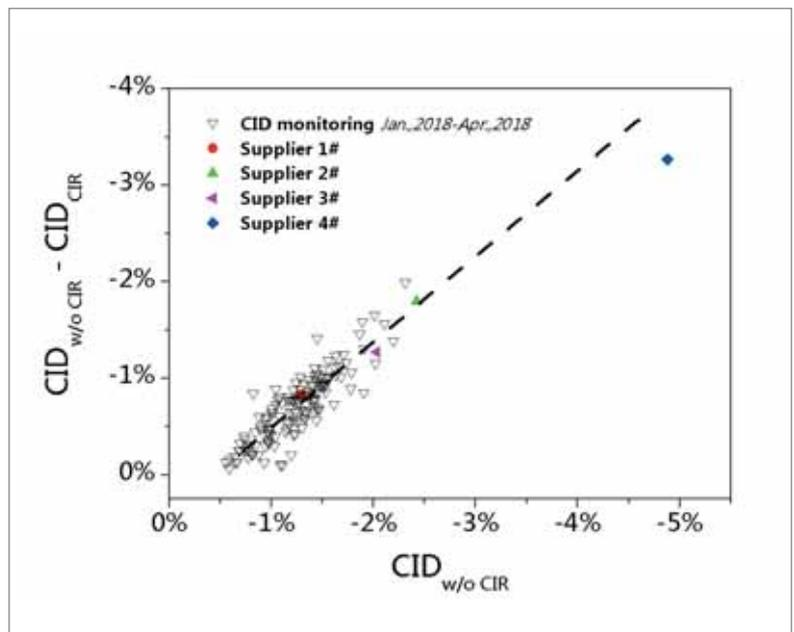
Figure 4. LID mitigation coefficient of the CIR process, reflected in the reduced degradation rate.
