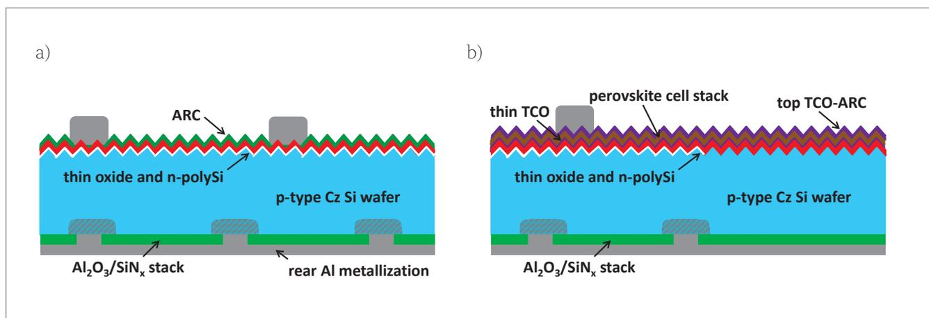
Figure 8. Schematic of the application of a polySi passivated contact in a bottom cell for a tandem stack in: (a) a PERC cell for 4T tandem application; (b) a possible 2T tandem layout based on the same cell concept.
