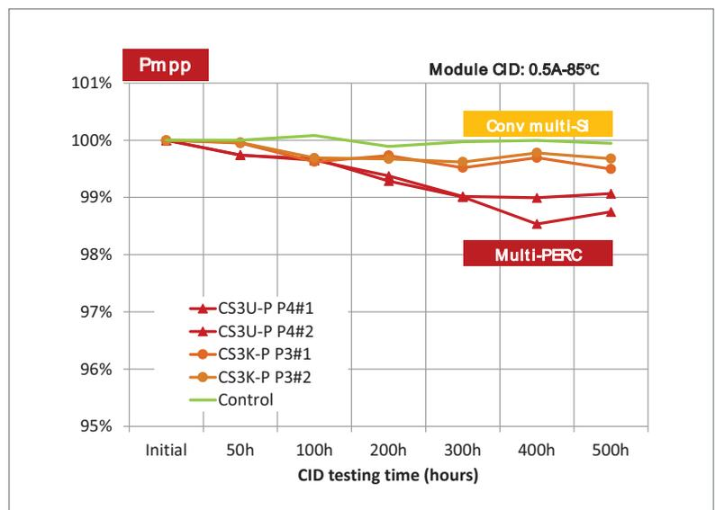
Figure 5. Module performance of CSI's multi-PERC modules undergoing CID testing.
