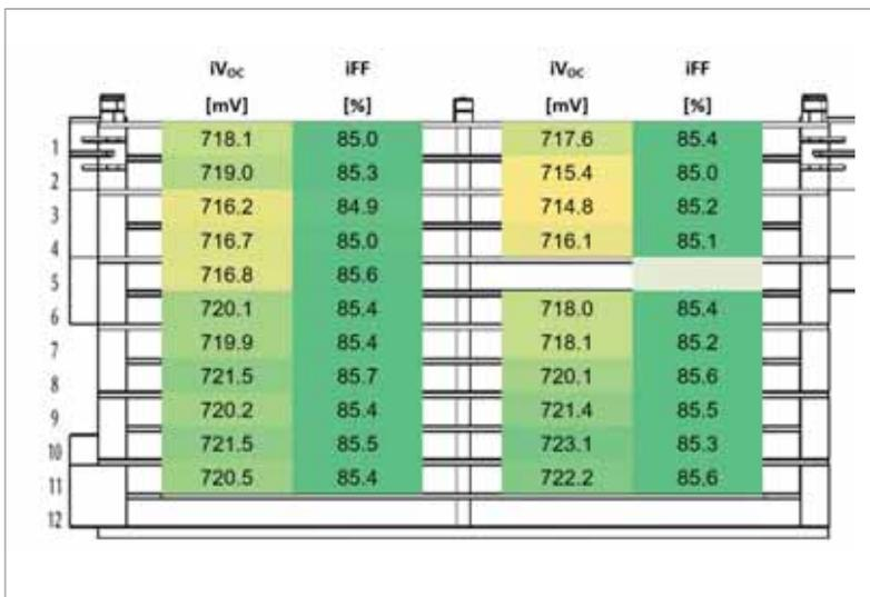
Figure 6. A side view of the PECVD carrier, listing the average  $iV_{oc}$  measured for each wafer [19].
