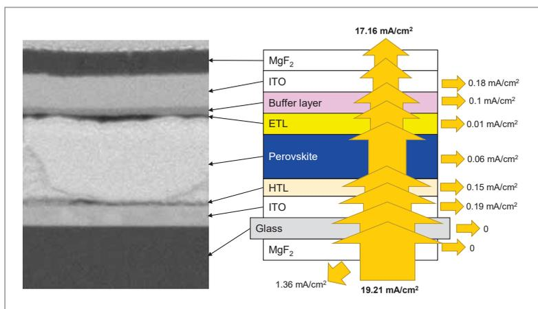
**Figure 2.** Cross-sectional scanning electron microscope (SEM) image of perovskite solar cell (left) developed at Solliance for use in 4T tandem cells, and its optical loss analysis (right) for the NIR region (800–1,200nm) of the AM1.5 spectrum (ETL = electron transport layer, HTL = hole transport layer) [9–11].
