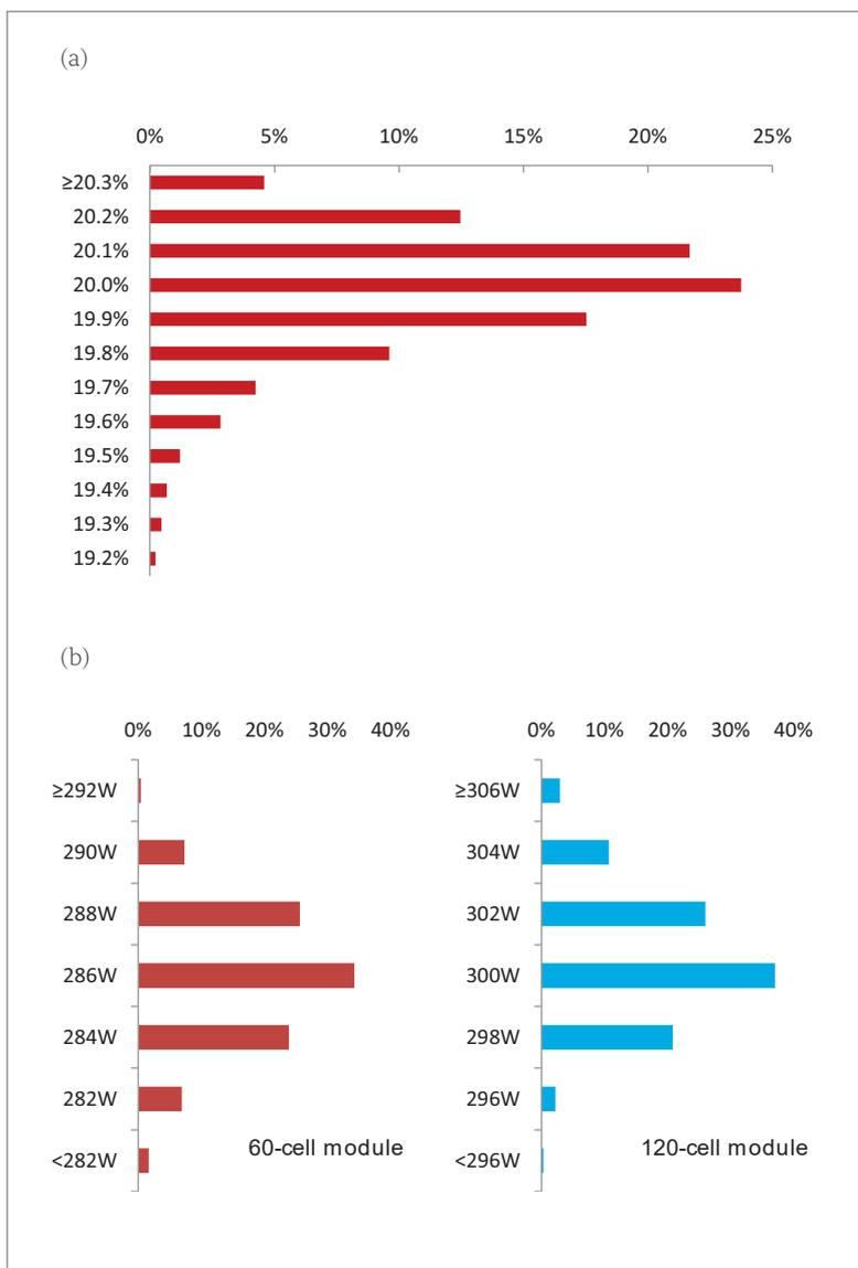
Figure 2. (a) Efficiency distribution of multi-PERC cells. (b) Wattage distribution of 60-cell and 120-cell multi-PERC modules.
