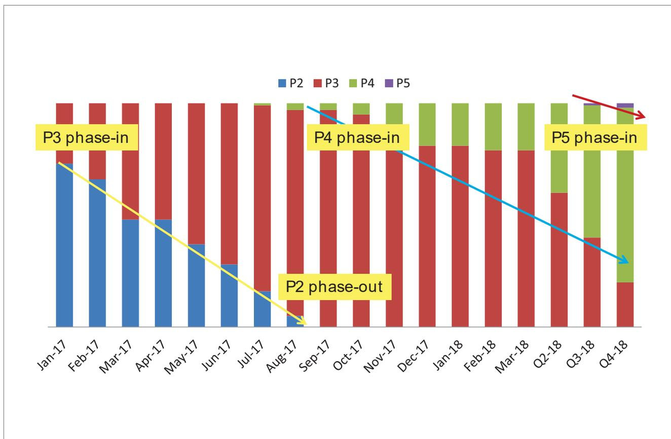
**Figure 6. Technology evolution of CSI's high-efficiency multi-Si product: P2 (conventional slurry), P3 (MCCE+DWS), P4 (multi-PERC), P5 (next-generation multi-Si).**
