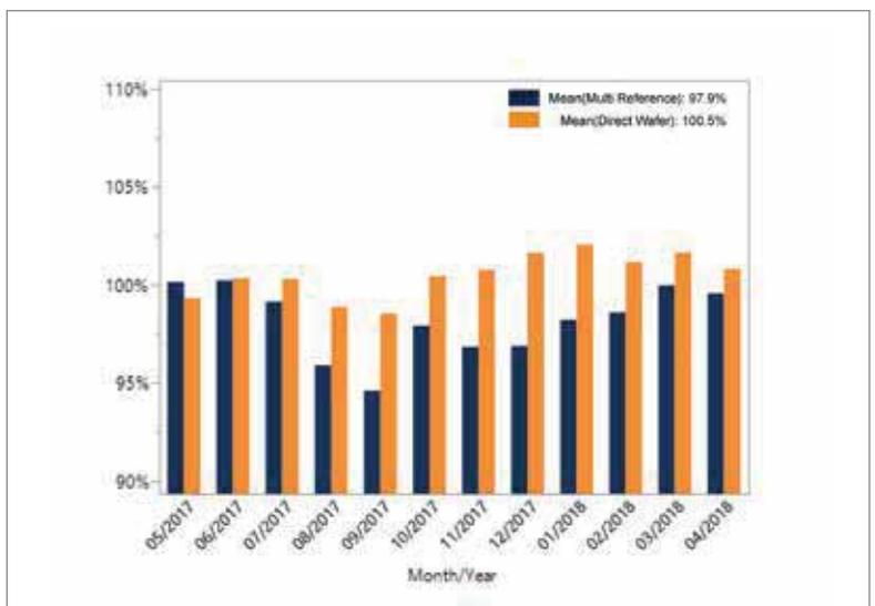
**Figure 11. Module performance of Direct Wafer modules at a commercial installation in Japan compared with HP mc-Si reference modules. Data was collected from the installation of more than 1,700 modules of each type.**
