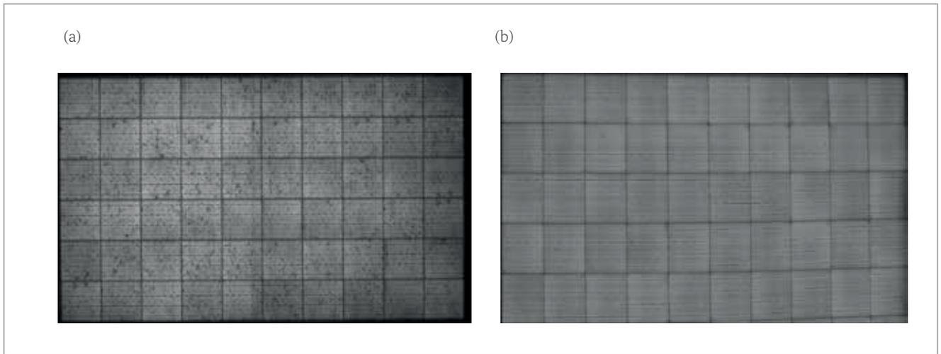
**Figure 9. EL images of PV modules made with (a) HP mc-Si wafers, and (b) Direct Wafer products. The impact of dislocation tangles is evident in multi.**
