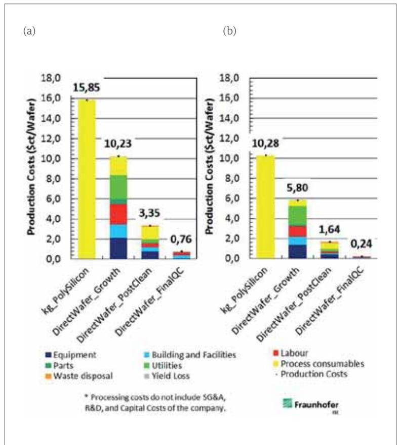
Figure 5. Direct Wafer net production costs (stepwise from left to right) for production with an annual output of (a) 1GWp (baseline), and (b) 10GWp (roadmap).
