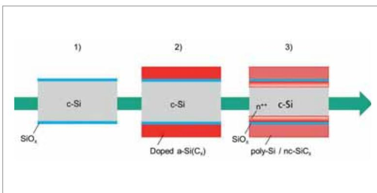
Figure 3. Steps involved in TOPCon fabrication: 1) interfacial oxide layer growth; 2) a-Si (or poly-Si) layer deposition; 3) high-temperature anneal.
